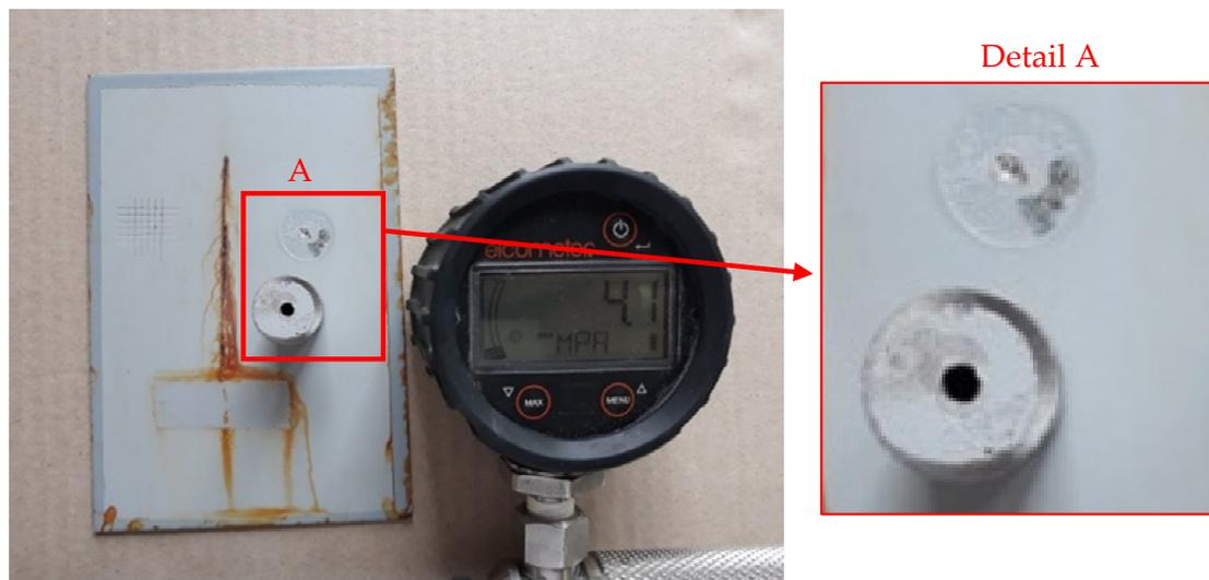
**Figure 2.** Specimen after the pull-off test.
