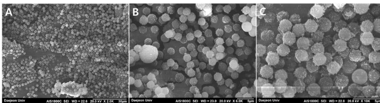
**Figure 3.** SEM images of microparticles of the top portion of PEG-DEX ATPS after the EDC coupling reaction with different magnifications. (A) 2000 times, (B) 6000 times, (C) 10,000 times magnified. Scale bars are (A) 30, (B) 5, (C) 5  $\mu\text{m}$ . See Experimental for other conditions.
