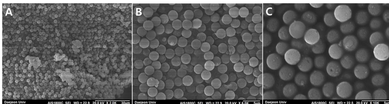
**Figure 5.** SEM images of microparticles of the bottom portion of PEG-DEX ATPS after the EDC coupling reaction with different magnifications. (A) 2000 times, (B) 6000 times, (C) 10,000 times magnified. Scale bars are (A) 30, (B) 5, (C) 5  $\mu\text{m}$ . See Experimental for other conditions.
