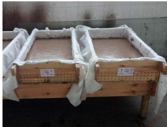
**Figure 6.** Soil sample remodeling.
