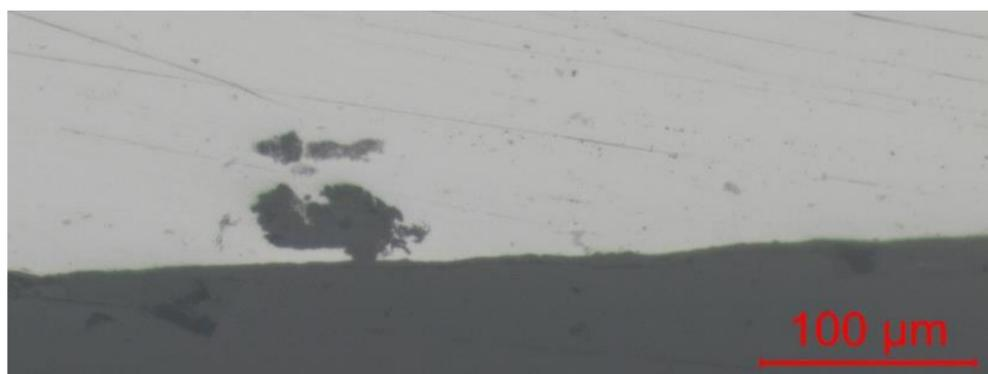
**Figure 1.** Pitting corrosion observed on AA 2050 T8.
