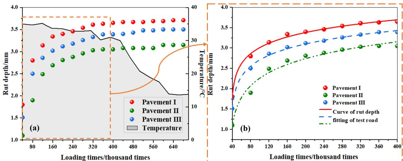
**Figure 8.** Variation law of pavement rutting. (a) Deformation curve of wheel rut section after 700,000 times of loading; (b) The overall evolution of the road ruts of the three different pavement structures under the action of loading and rolling at room temperature.
