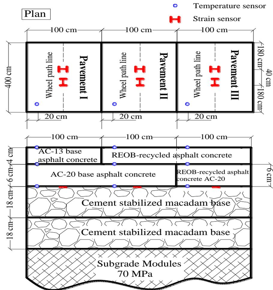
Figure 4. Road structure and sensor location map.
