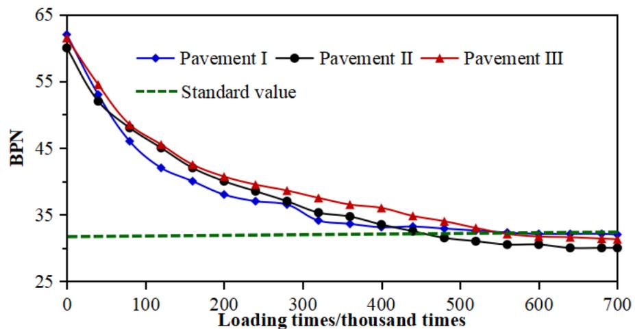
Figure 7. Variation law of pavement friction coefficient.
