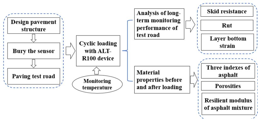
Figure 3. Flow chart of the accelerated loading test.
