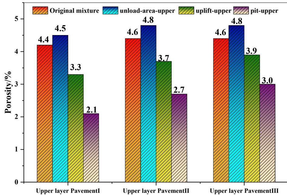
Figure 12. Porosities of cores taken from different pavements.
