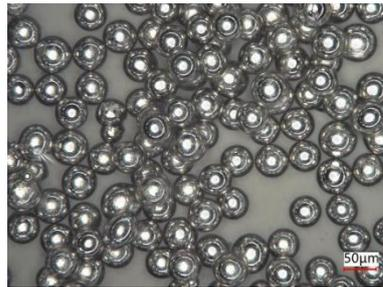
**Figure 11.** Microscopic image of Inconel718 alloy powder.
