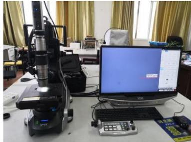
**Figure 10.** Super-depth-of-field microscope.
