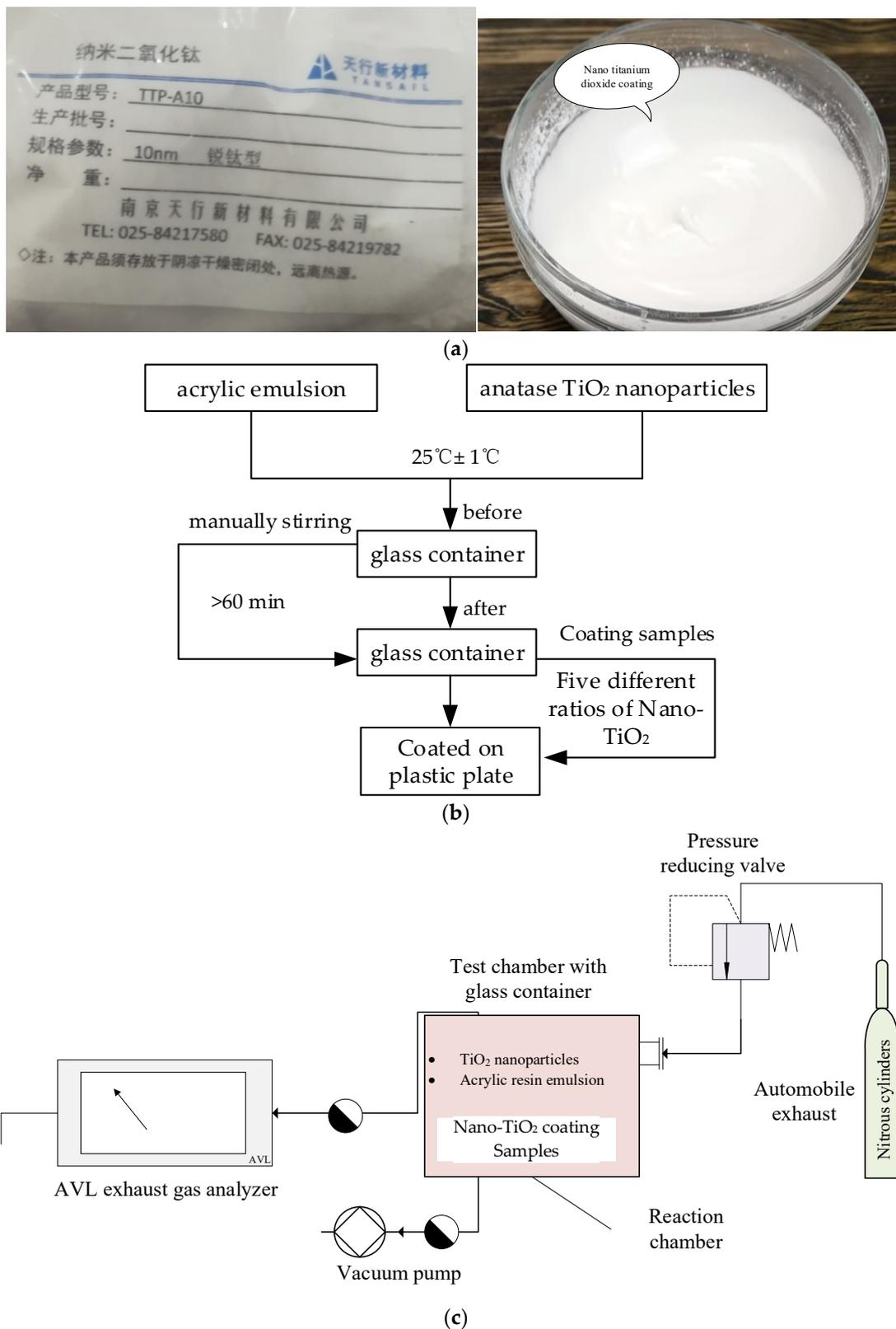
**Figure 4.** Test devices and mixing process for degradation effect of nano-TiO<sub>2</sub> coating material. (a) Critical materials (Left: anatase Nano-TiO<sub>2</sub> particles; Right: Nano-TiO<sub>2</sub> coatings). (b) Mixing process flowchart of coating samples. (c) Devices connection in the laboratory.
