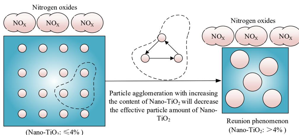
Figure 8. Nano-TiO<sub>2</sub> agglomeration for decreasing the catalytic speed.
