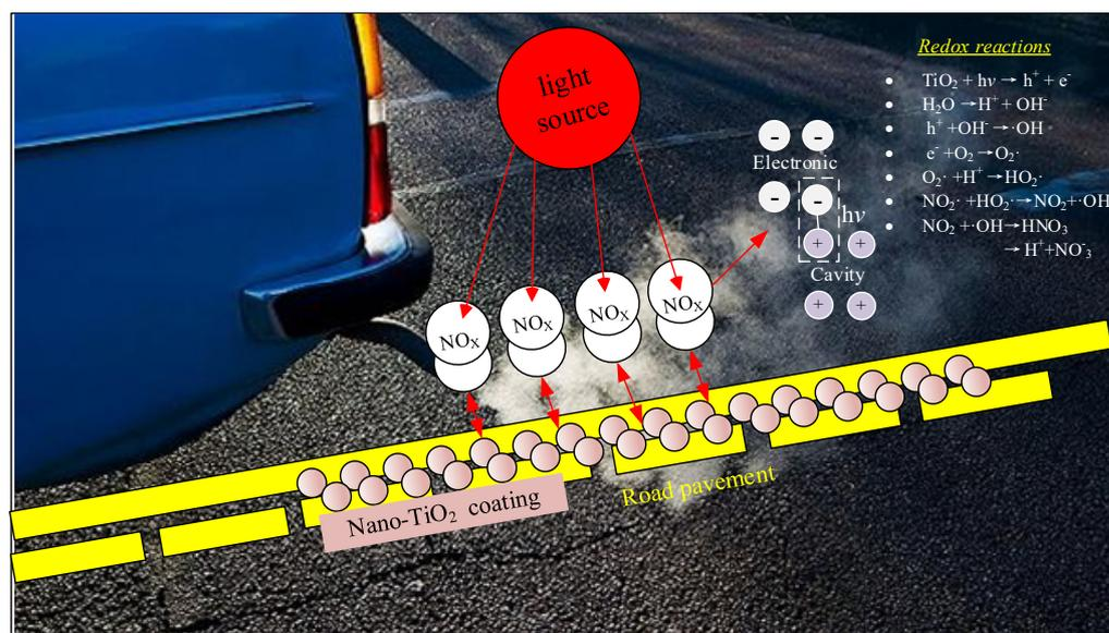
Figure 3. Catalytic principle of Nano- $\text{TiO}_2$  coatings.
