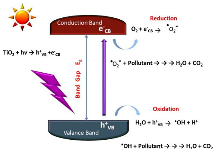
**Figure 2.** Mechanism of TiO<sub>2</sub> photocatalysis [23].
