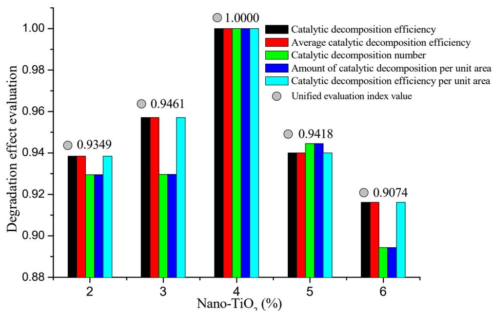
Figure 7. Effect of the coating degradation.
