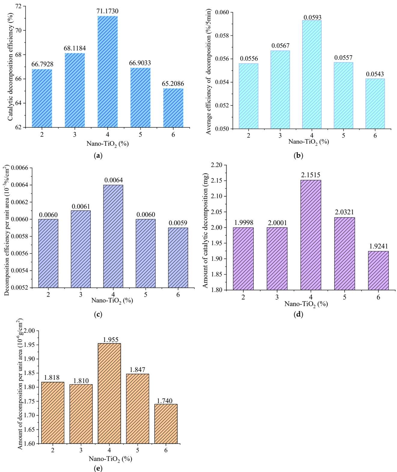
**Figure 6.** Catalytic evaluations with different contents of Nano-TiO<sub>2</sub>. (a) Catalytic decomposition efficiency (C). (b) Average catalytic efficiency (V<sub>c</sub>). (c) Decomposition efficiency per unit area (e). (d) Amount of catalytic decomposition (m). (e) Amount of decomposition per unit area (d).
