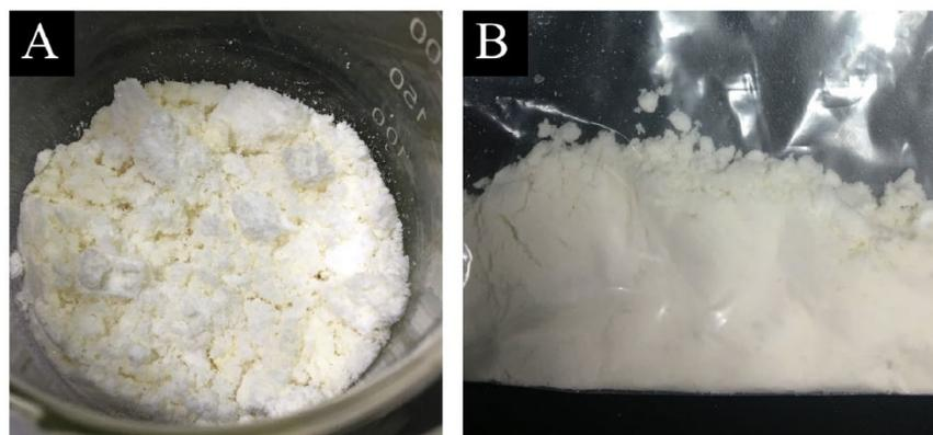
**Figure 2.** Macro morphology of the microcapsules: (A) the microcapsules before grinding, (B) the microcapsules after grinding.
