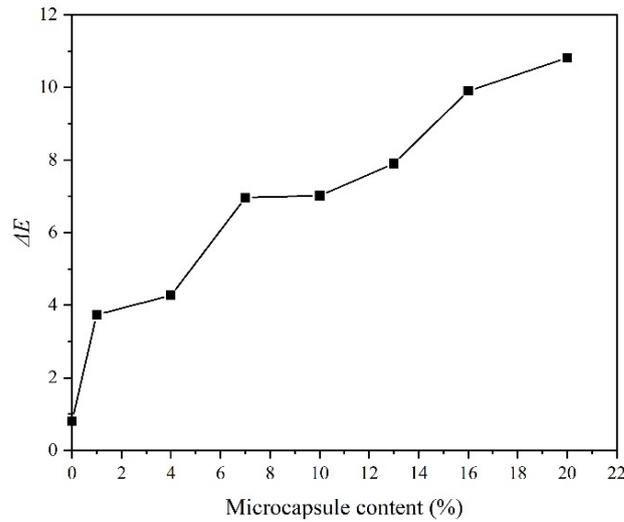
Figure 6. Effect of the microcapsule content on color difference of the coatings.
