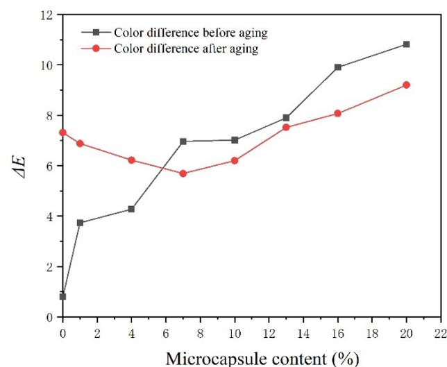
**Figure 11.** Effect of the microcapsule content on color difference of the coatings before and after aging.
