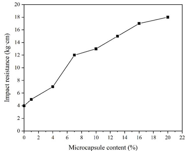
**Figure 10.** Impact resistance of coatings.
