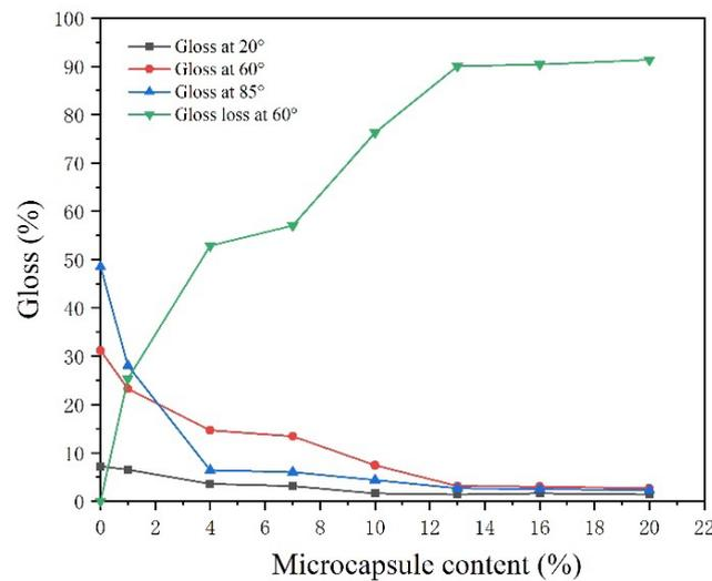
Figure 7. Effect of the microcapsule content on gloss of the coatings.
