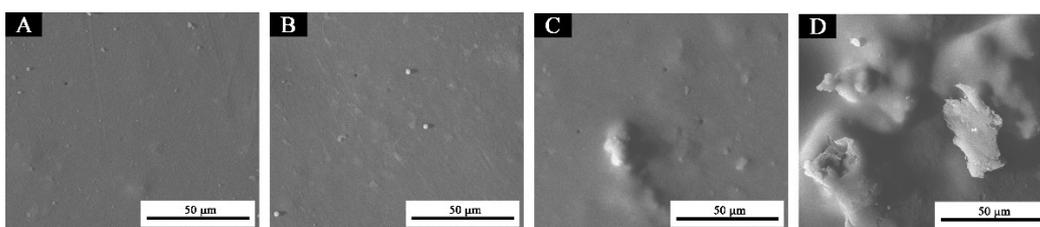
Figure 4. Morphology of the coatings with different content of the microcapsules: (A) 0%, (B) 1.0%, (C) 7.0%, (D) 13.0%.
