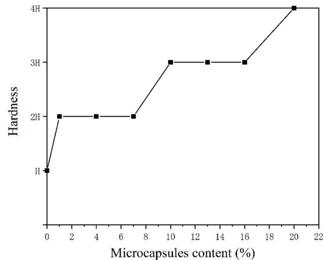
**Figure 8.** Hardness of the coatings.
