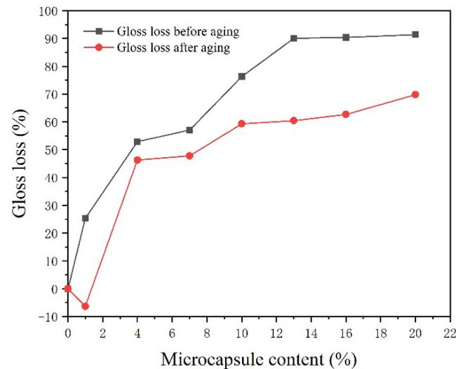
**Figure 12.** Effect of the microcapsule content on gloss loss of the coatings before and after aging.
