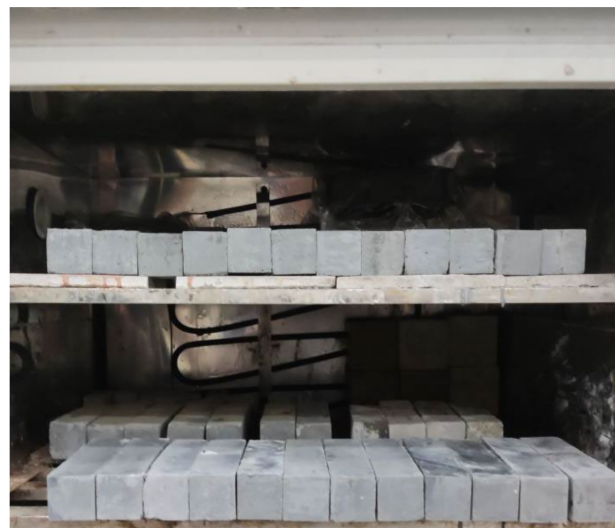
Figure 4. UHPC in the standard curing chamber.
