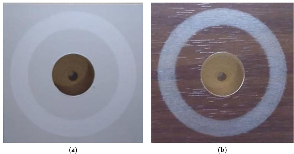
**Figure 7.** The surface finish after abrasion: (a) PVC foil, gloss; (b) PVC foil, matte.
