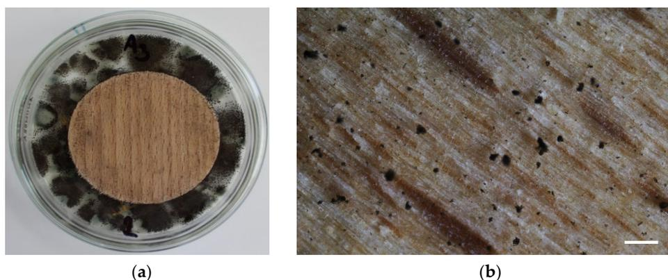
**Figure 5.** The evaluated resistance-to-mould growth: (a) sample in glass dishes; (b) mould growth on surface of test sample treated with transparent natural wax with oil (scale bar = 1 mm).
