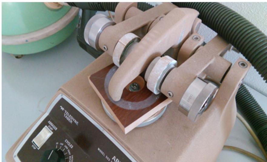
**Figure 3.** The evaluated resistance-to-abrasion in the Taber abrasion tester model 503.
