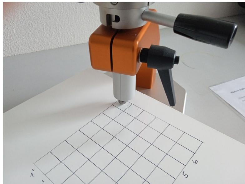
**Figure 2.** The impact resistance measured by falling weight impact tester.
