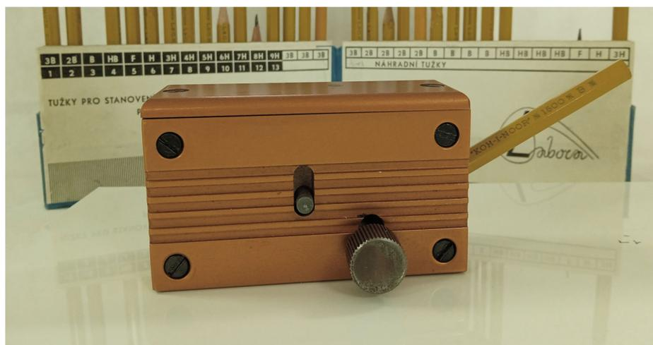
**Figure 1.** The pencils of different degrees of hardness and the preparation with a weight of 300 g.
