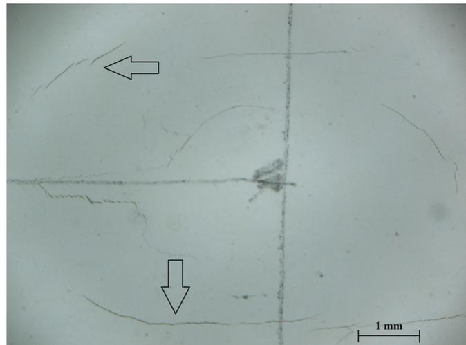
**Figure 6.** Cracking visible on the surfaces with pigmented surface finish (pigment, matte, 4 layers) after impact resistance testing at the drop height of 400 mm (visible at magnification 17×).
