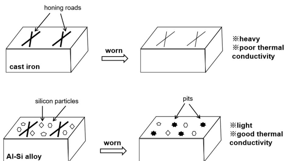
Figure 13. Schematic diagram of the cylinder liner wear process.
