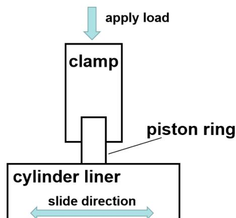
**Figure 3.** Schematic diagram of reciprocating-wear tests.
