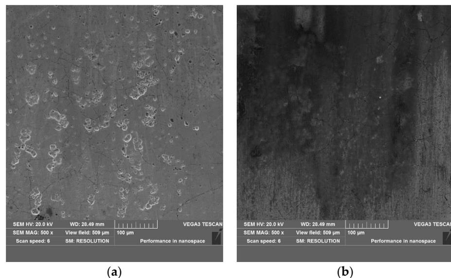
**Figure 12.** Scuffing surface morphology of piston ring (SEM): (a) CKS piston ring worn against cast-iron cylinder liner; (b) CKS piston ring worn against Al-Si alloy cylinder liner.
