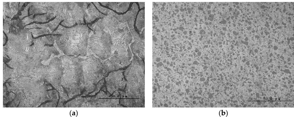
**Figure 2.** Polished surface of cylinder liners. (a) Cast-iron cylinder liner. (b) Al-Si alloy cylinder liner.
