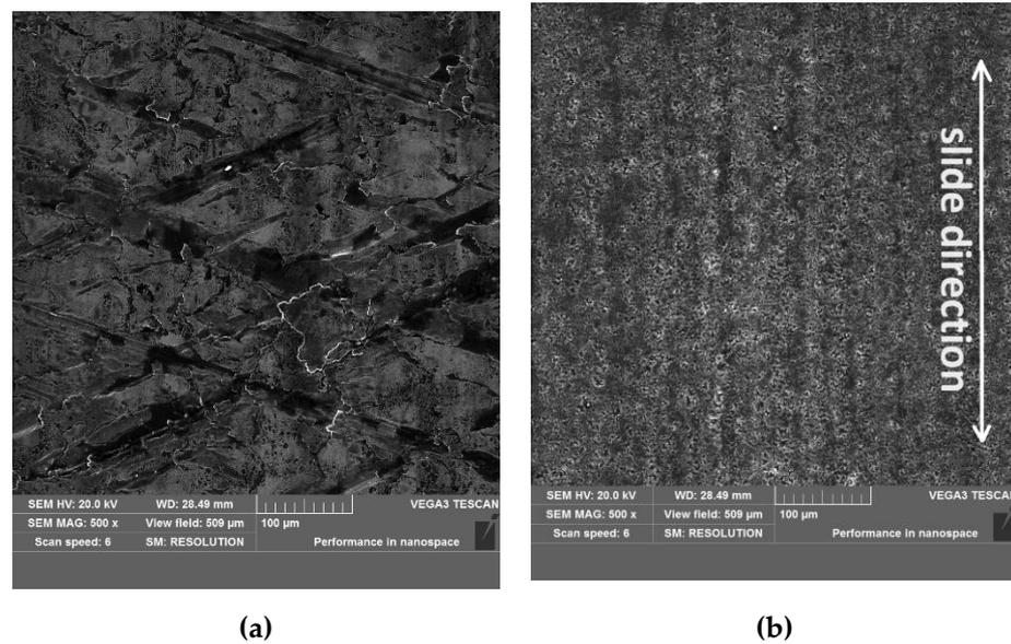
**Figure 7.** Worn surface morphology of cylinder liners: (a) cast-iron cylinder liner; (b) Al-Si alloy cylinder liner.
