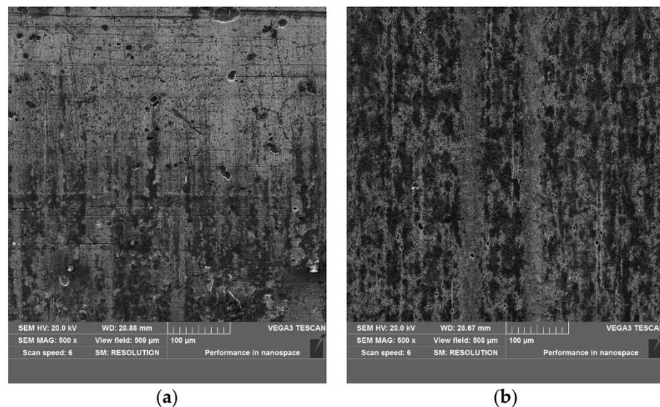
**Figure 8.** Worn surface morphology of CKS piston ring (SEM): (a) CKS piston ring worn against cast-iron cylinder liner; (b) CKS piston ring worn against Al-Si alloy cylinder liner.
