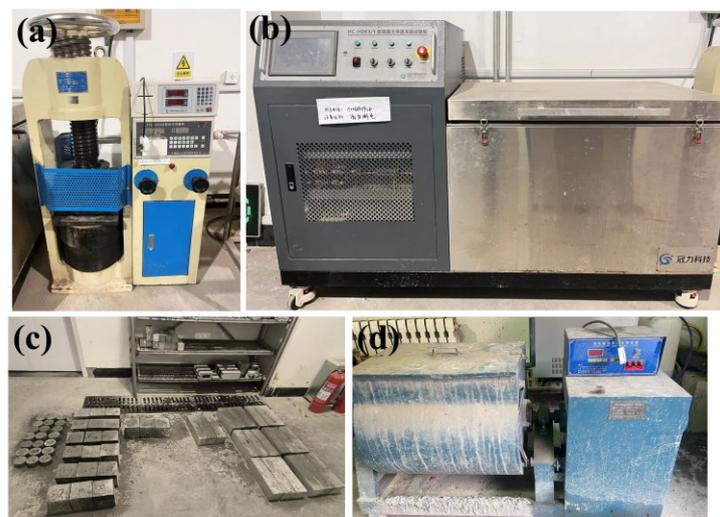
**Figure 2.** Experimental instruments and samples: (a) Pressure testing machine, (b) concrete rapid freeze–thaw tester, (c) various specimens, (d) concrete mixer.
