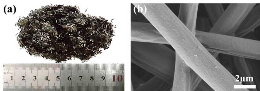
**Figure 1.** The photo and SEM image of carbon fiber. The photo (a) and SEM (b) image of carbon fiber.
