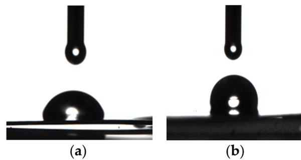
**Figure 3.** Contact angle of (a) 316 stainless steel and (b) Ni–P–TiO<sub>2</sub>.
