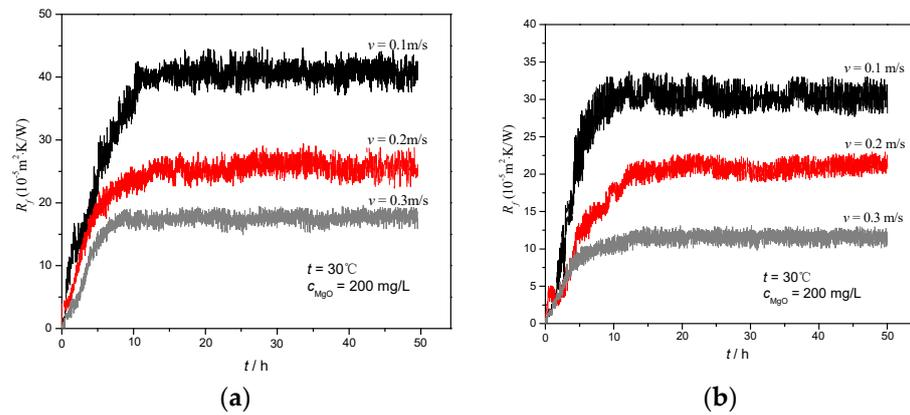
**Figure 7.** Influence of cooling water velocity on the fouling heat resistance of (a) 316 stainless steel plate and (b) Ni–P–TiO<sub>2</sub> composited coating.
