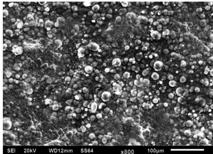
Figure 1. Morphology of Ni–P–TiO<sub>2</sub> composite coating.
