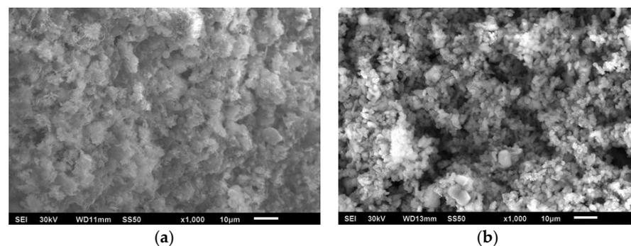
**Figure 6.** Microtopography of particulate fouling deposition on (a) the 316 stainless steel and (b) the Ni–P–TiO<sub>2</sub> composite coating.
