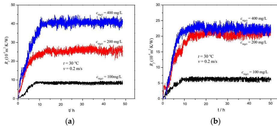
**Figure 10.** Influence of MgO nanoparticle concentration on the fouling resistance of (a) 316 stainless steel plate and (b) Ni–P–TiO<sub>2</sub> composited coating.
