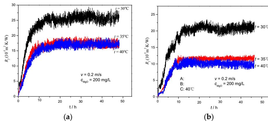
**Figure 9.** Influence of cooling water temperature on the fouling resistance of (a) 316 stainless steel plate and (b) Ni–P–TiO<sub>2</sub>–composited coating.
