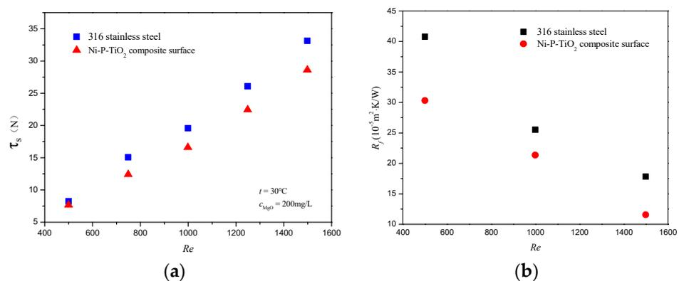
**Figure 8.** Influence of fluid velocity on (a) the wall shear force and (b) the fouling resistance asymptotic value.
