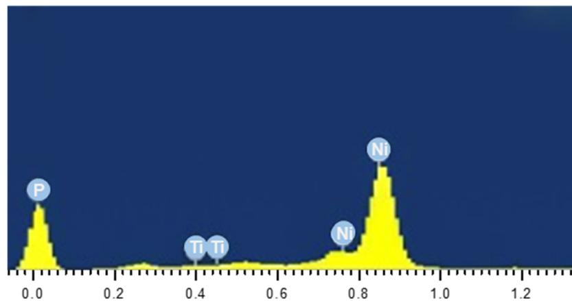
Figure 2. Element analysis of Ni–P–TiO<sub>2</sub> composite coating.
