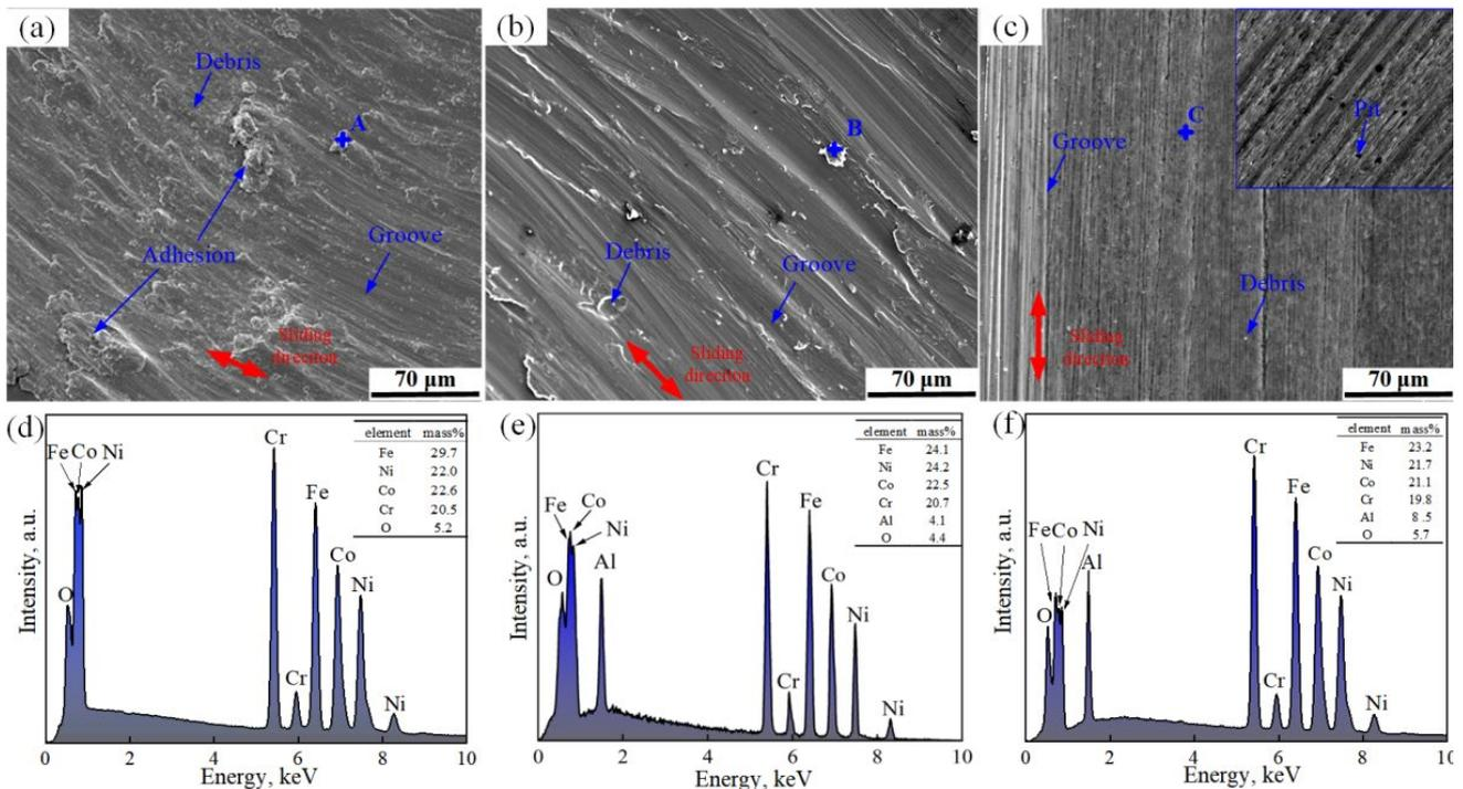
Figure 8. SEM images of worn surfaces and elements of the coatings of (a,d) FeCoCrNi, (b,e) FeCoCrNiAl<sub>0.5</sub>, (c,f) FeCoCrNiAl.
