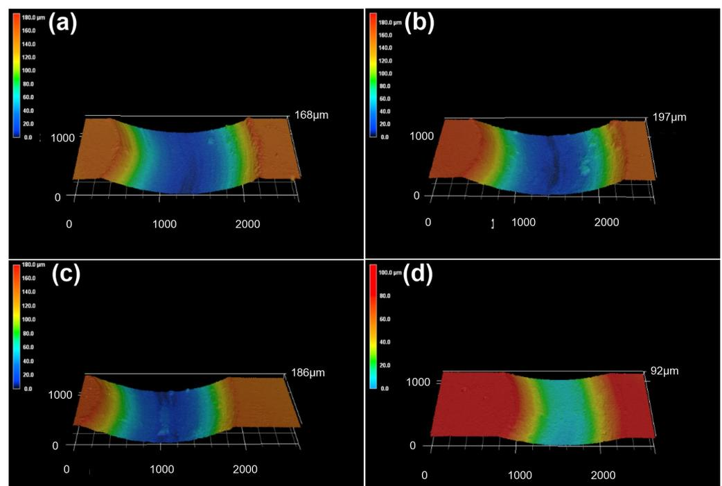
**Figure 9.** 3D morphologies of the worn surfaces of the (a) substrate, (b) FeCoCrNi, (c) FeCoCrNiAl<sub>0.5</sub>, (d) FeCoCrNiAl.
