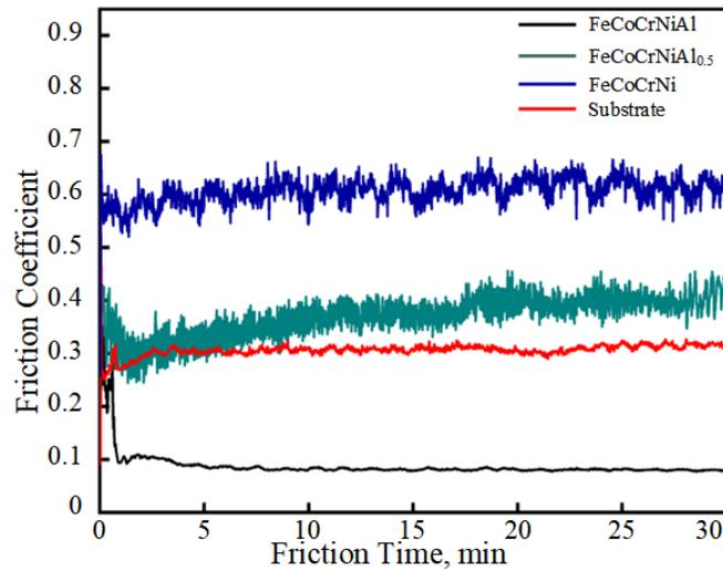
Figure 7. Coefficients of friction of the coatings with different Al contents.
