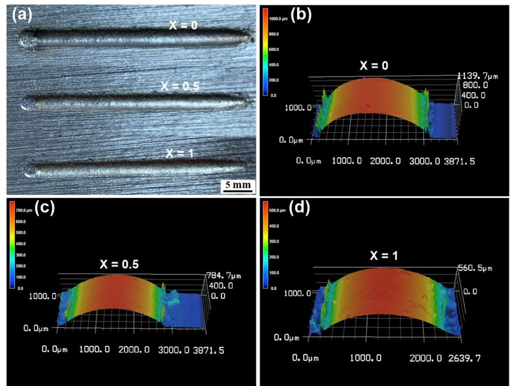
**Figure 2.** 3D morphologies of FeCoCrNiAl<sub>x</sub> single cladding tracks with different Al contents. (a) morphologies of tracks, (b–d) the reconstructed 3D morphologies of tracks with different Al contents.
