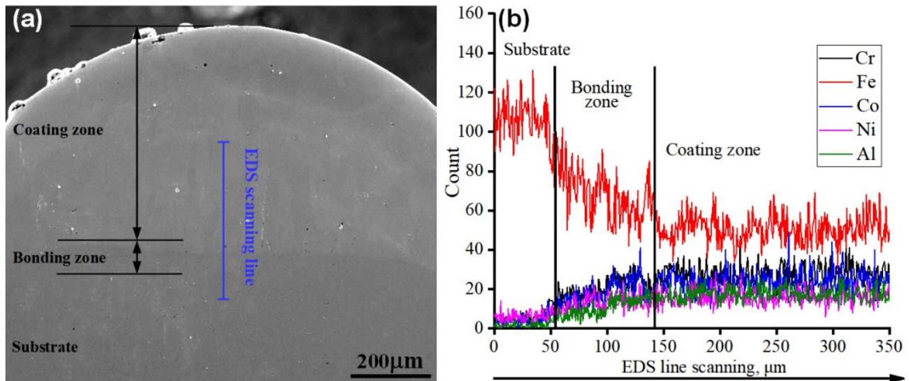
**Figure 3.** (a) SEM morphology of cross-section of the FeCoCrNiAl single cladding track, and (b) element distribution along the height direction.
