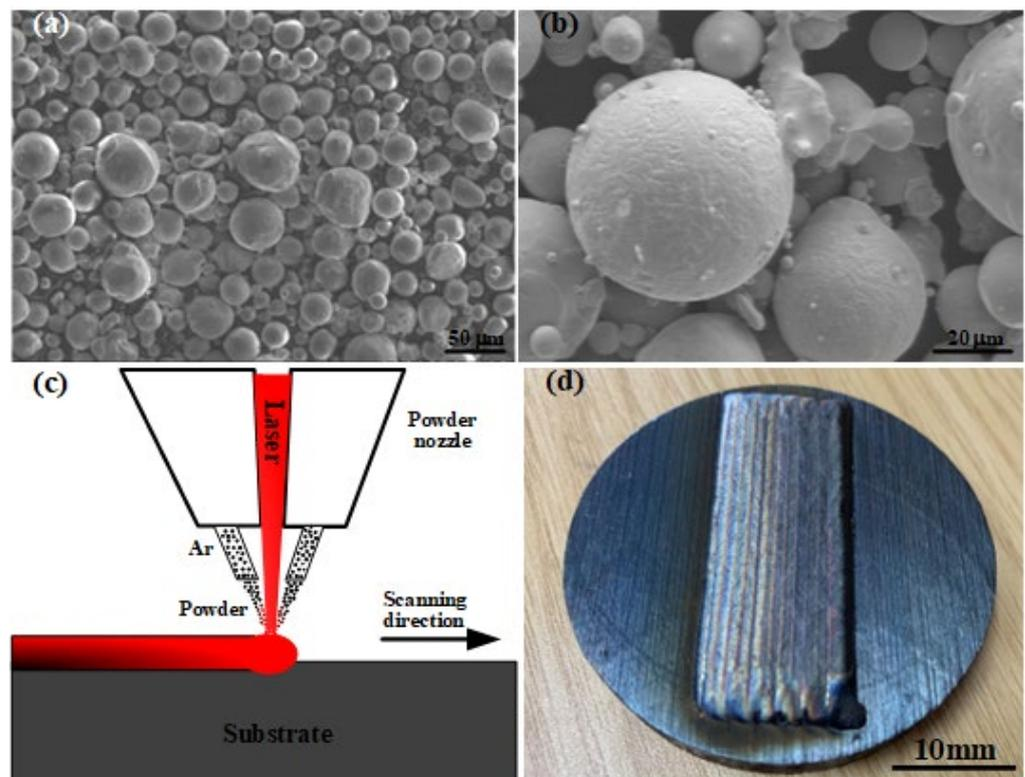
**Figure 1.** (a,b) Morphology of FeCoCrNiAl HEA powder, (c) schematic diagram of laser cladding process, (d) FeCoCrNiAl HEA coating.
