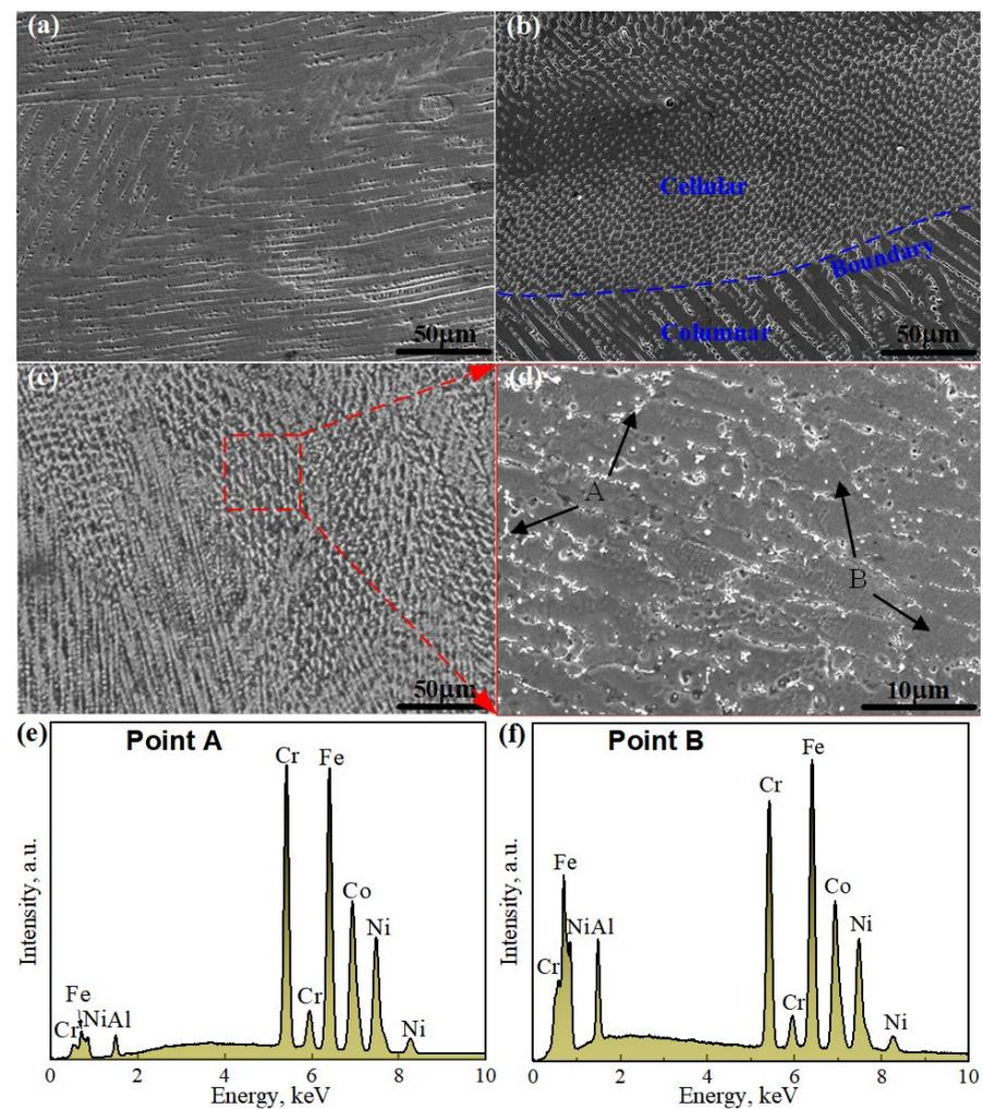
**Figure 5.** SEM images of cross-sections of single cladding tracks of (a) FeCoCrNi, (b) FeCoCrNiAl<sub>0.5</sub>, (c,d) FeCoCrNiAl, (e,f) EDS of points A and B indicated in (d).
