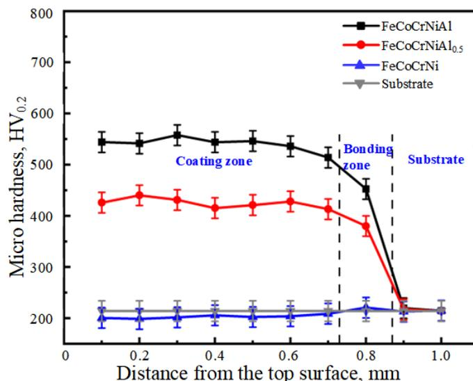
**Figure 6.** Micro hardness of single cladding tracks from coating top surface to substrate, the distance between the measuring points is about 100 mm.
