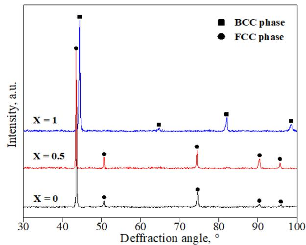
**Figure 4.** XRD patterns of the coatings with different Al contents.
