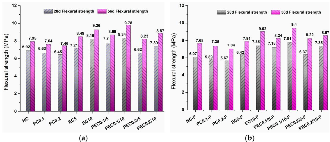
Figure 7. Flexural strength of different types of concrete: (a) OPC; (b) 90% OPC + 10% FA.
