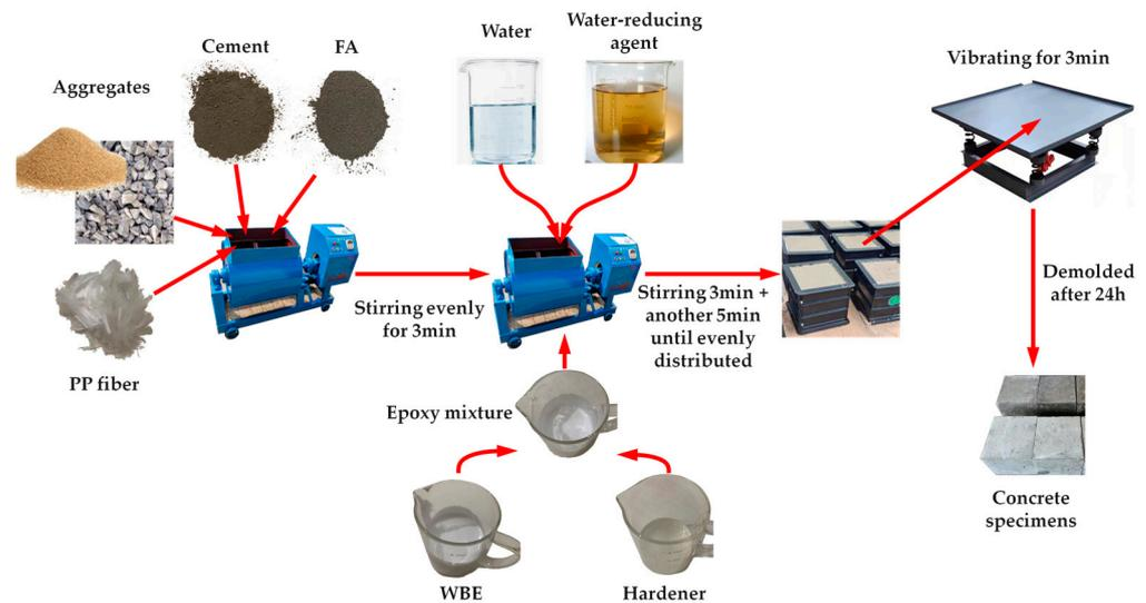
**Figure 1.** Graphical procedure of concrete specimen preparation.
