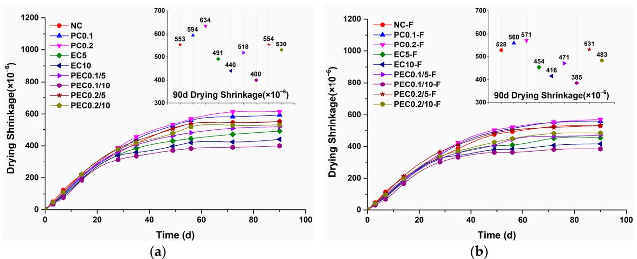
Figure 8. Drying shrinkage of different types of concrete: (a) OPC; (b) 90% OPC + 10% FA.
