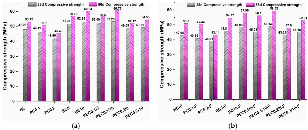
Figure 3. Compressive strength of different types of concrete: (a) OPC; (b) 90% OPC + 10% FA.
