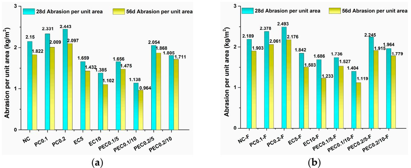
Figure 10. Abrasion per unit area of different types of concrete: (a) OPC; (b) 90% OPC + 10% FA.
