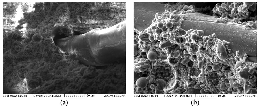
**Figure 6.** Microstructural images of different types of concrete with FA by SEM: (a) PC0.1-F; (b) PEC0.1/10-F.
