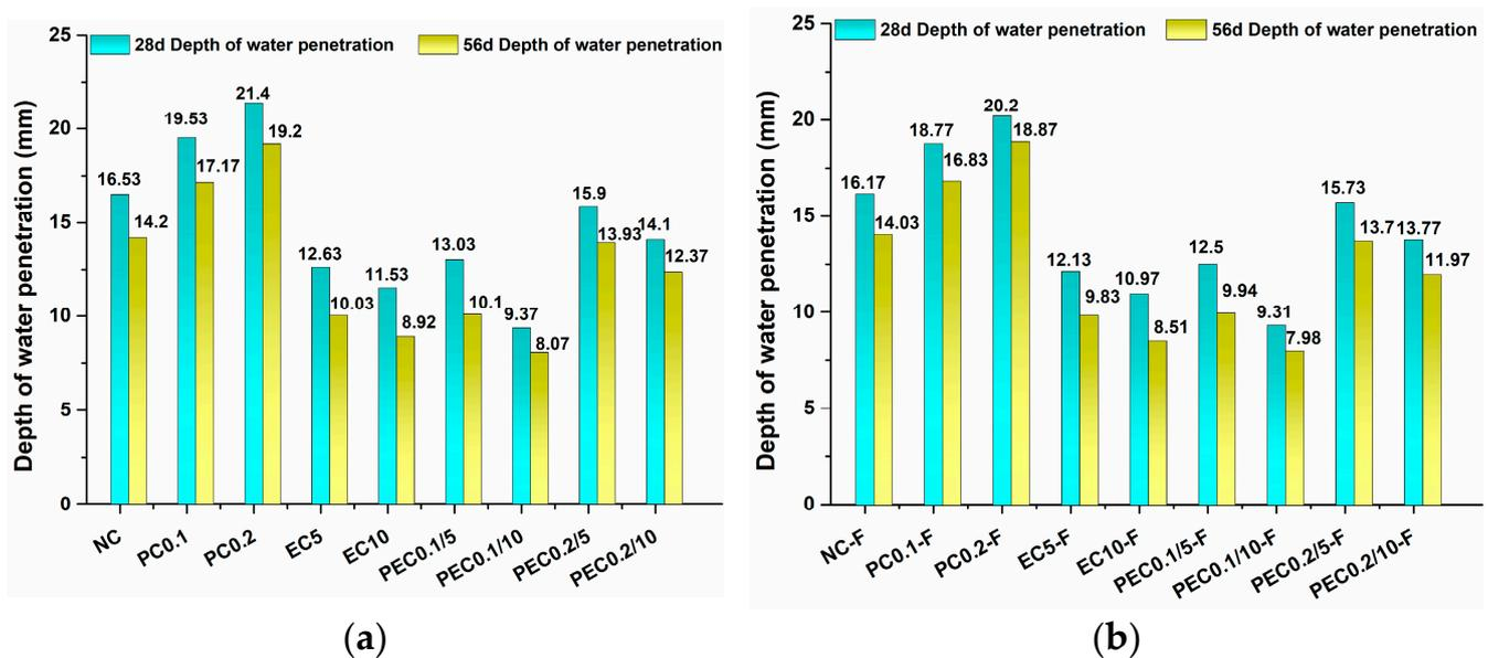
Figure 9. Depth of water penetration of different types of concrete: (a) OPC; (b) 90% OPC + 10% FA.
