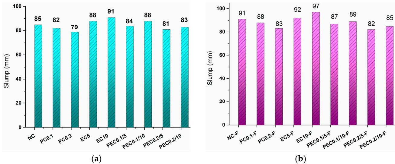
Figure 2. Slump of different types of concrete: (a) OPC; (b) 90% OPC + 10% FA.
