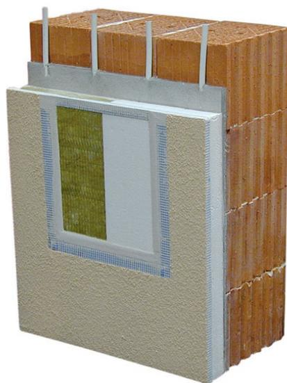
**Figure 4.** Application of TB on a brick wall [5].
