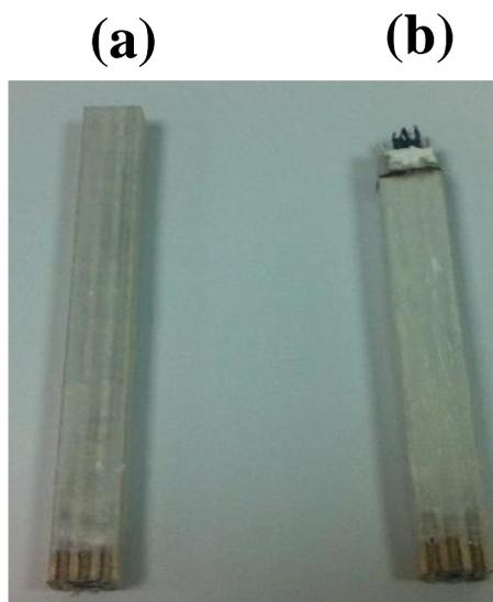
**Figure 3.** Plywood specimens prepared for LOI measurements. Unburned specimen coated with (a) polymer matrix/H5/additive and (b) burned specimen.
