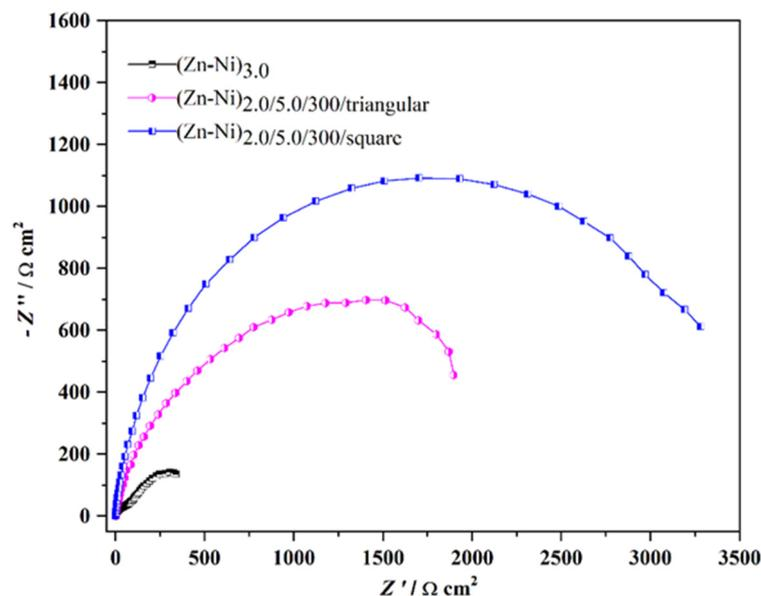
Figure 5. Electrochemical impedance spectra of single-layer and multilayer coatings.
