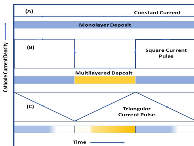
**Figure 1.** Graphical depiction of waveforms of single-layer (A) multilayer using square (B) and triangular current pulses (C).
