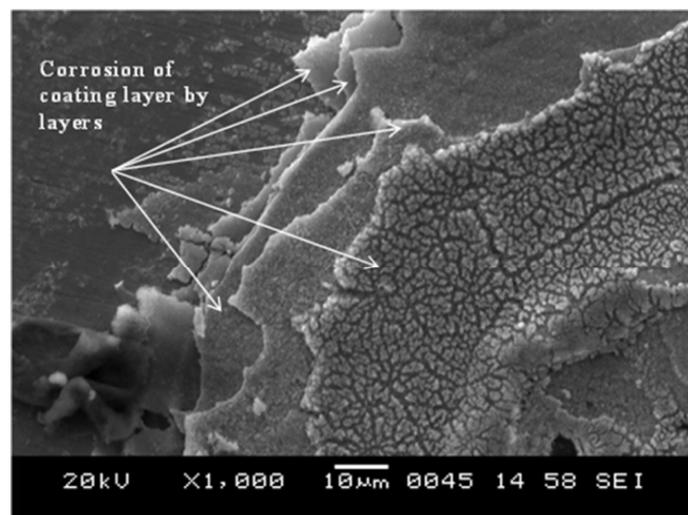
Figure 9. SEM image of multilayer electroplating after the corrosion analysis:  $(\text{Zn-Fe})_{3/5/4/\text{square}}$ .
