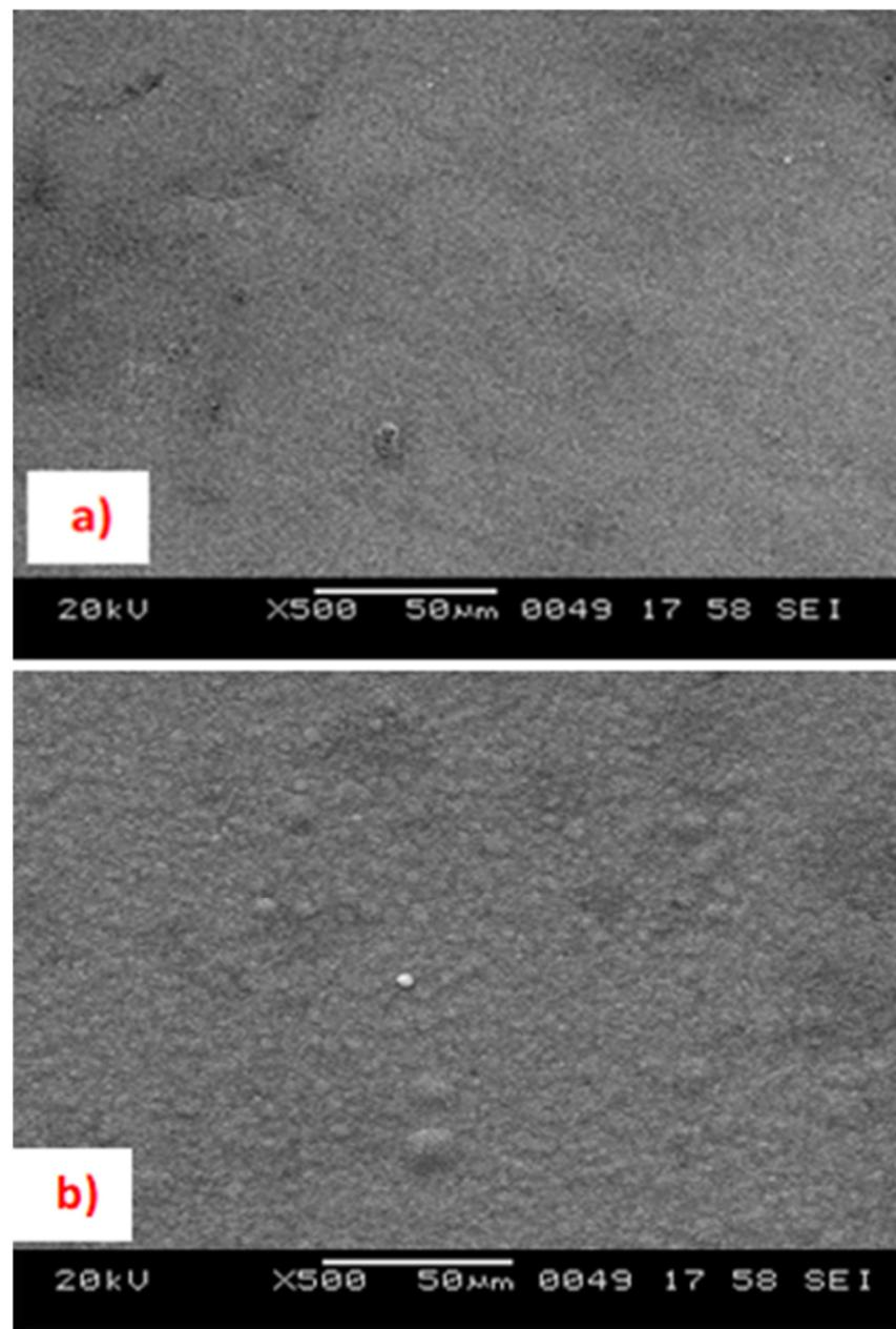
**Figure 7.** Surface topography of Zn-Fe multilayer coatings by the square (a) and triangular (b) current pulses.
