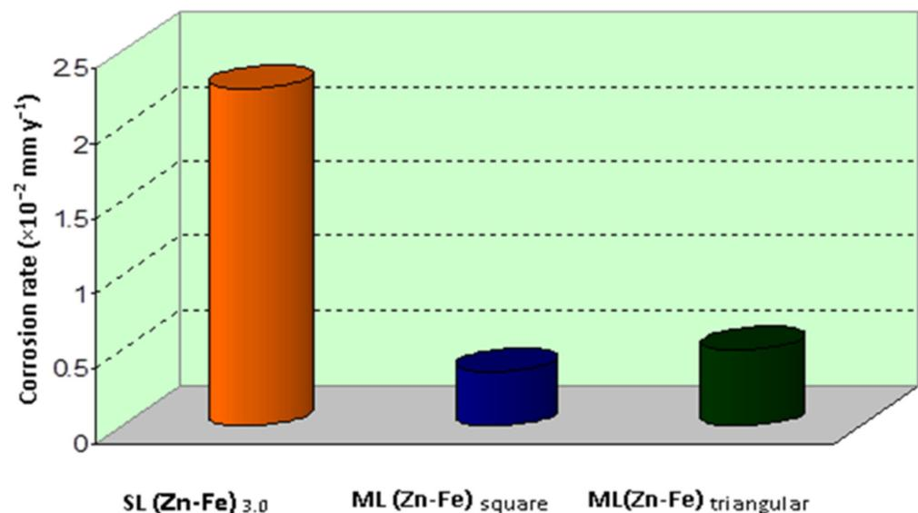
Figure 4. Relative analysis of corrosion rate of single-layer and ML alloy films.
