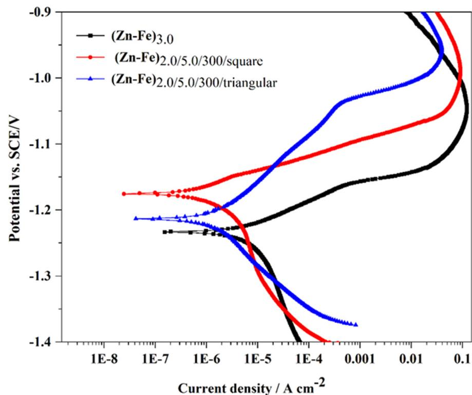
**Figure 3.** Potentiodynamic polarization curves of SL and ML alloy deposits.
