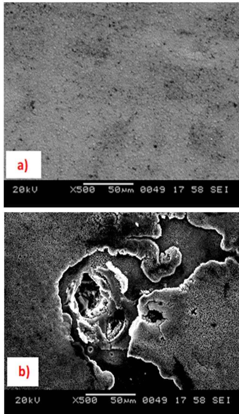
**Figure 6.** Surface topography of single-layer Zn-Fe alloy electroplating (a); the surface after corrosion test (b).
