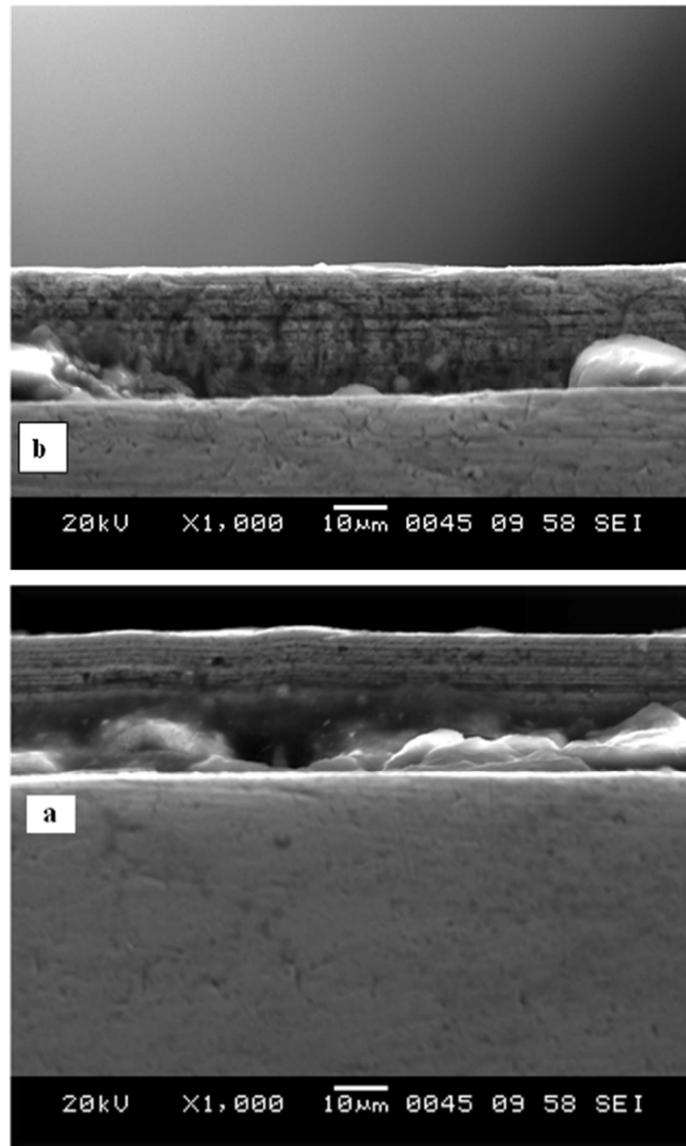
Figure 8. Cross-sectional images of multilayer Zn-Fe deposits with square (a) and triangular (b), pulses.
