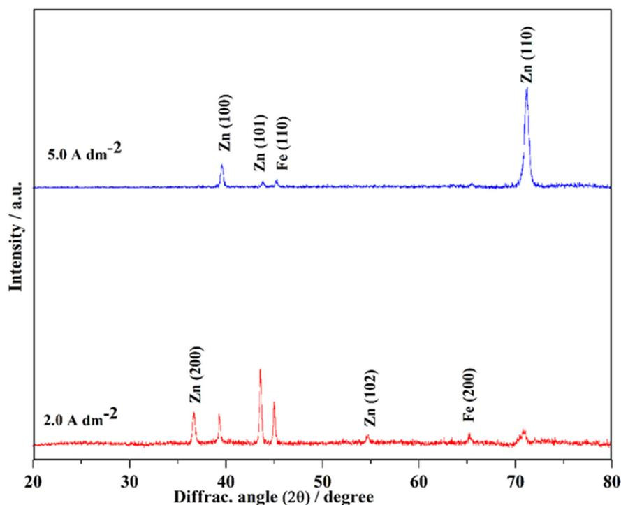
**Figure 2.** X-ray diffraction profiles of Zn-Fe alloy electroplate on MS developed from the optimized bath at  $i = 3.0$  and  $5.0 \text{ A dm}^{-2}$ .
