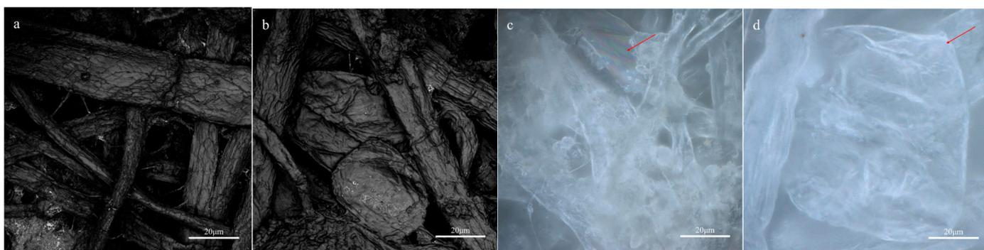
**Figure 9.** The morphology of paper was observed by laser microscope. (a) Laser image of unreinforced paper fibers; (b) Laser image of reinforced paper fibers; (c) Color image of reinforced paper fibers cross-linking; (d) Color image of the colloidal particles between reinforced paper fibers.
