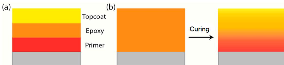
**Figure 5.** (a) A normal three-coat system; (b) a self-stratifying coating system as sprayed (left) and drying over time (right).
