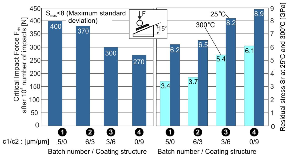
**Figure 8.** The determined data for the investigated CDCs with various structure architectures.
