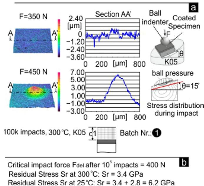
**Figure 7.** (a) Formation of a coating bulge due to interface fatigue failure during the inclined impact test in the examined 1st batch case; (b) calculation of the overall residual stresses in the film structure at 300 °C and 25 °C.
