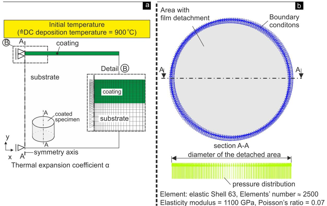
**Figure 3.** (a) The developed FE model used to calculate thermal residual stresses after the film cooled from the deposition temperature to operational one; (b) the developed FE model used to simulate the coating bulge geometry.
