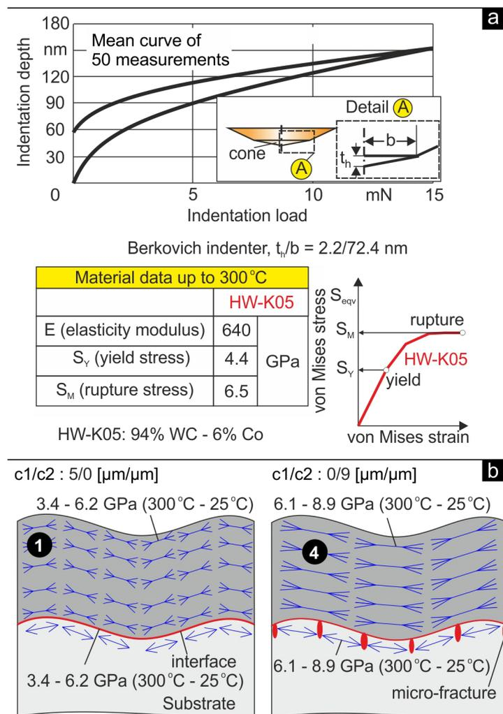
**Figure 10.** (a) Substrate material mechanical properties; (b) coating interface failure due to exceed of the substrate rupture stress caused by high residual stresses.
