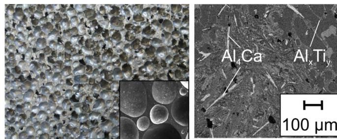
Workpiece material: Aluminium foam
