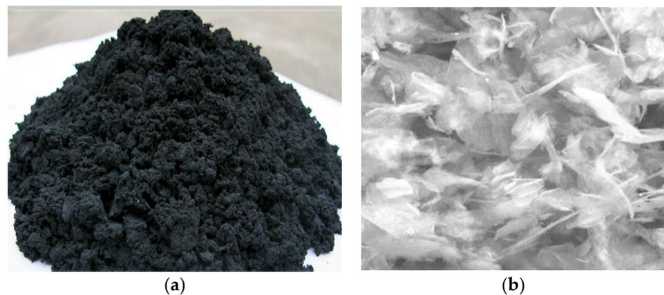
**Figure 3.** Graphene modifier. (a) Graphene powder, (b) Graphene under SEM.
