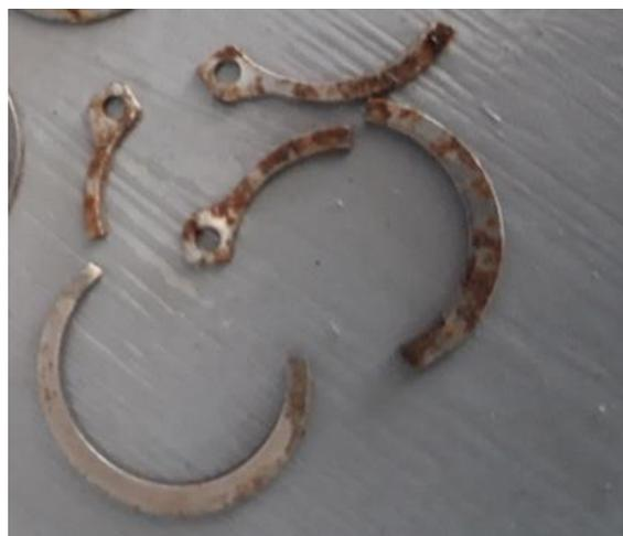
**Figure 6.** Examples of stress corrosion cracked snap rings.
