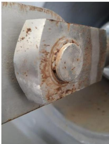
**Figure 7.** Detail of the support roller showing the snap ring located in a carved narrow groove. Localized corrosion and rusting are shown.
