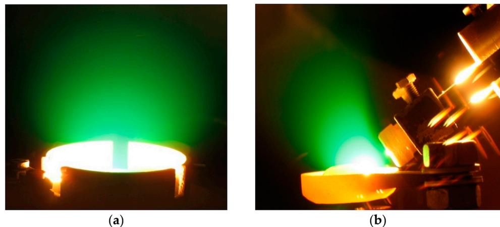
**Figure 44.** Copper TVD plasmas. (a) Ring cathode structure; (b) electron gun structure.
