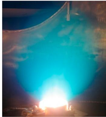
**Figure 53.** The nickel TVD plasma image, generated with ring cathode geometry.
