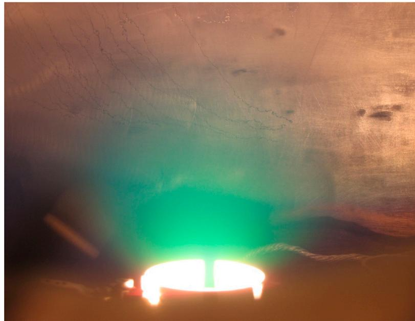
Figure 48. The silver TVD plasma image with ring cathode arrangement.
