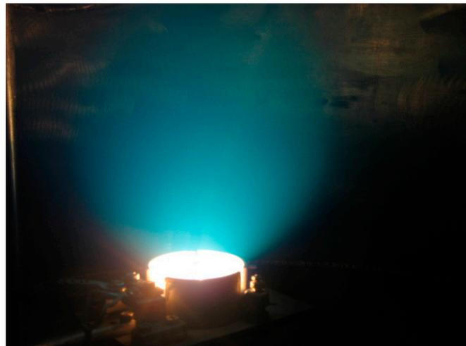
**Figure 57.** Chromium TVD plasma image generated in the ring cathode geometry.
