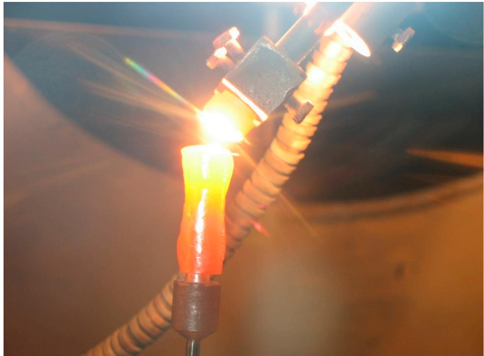
**Figure 38.** Rhenium deposition from a rhenium anode rod.
