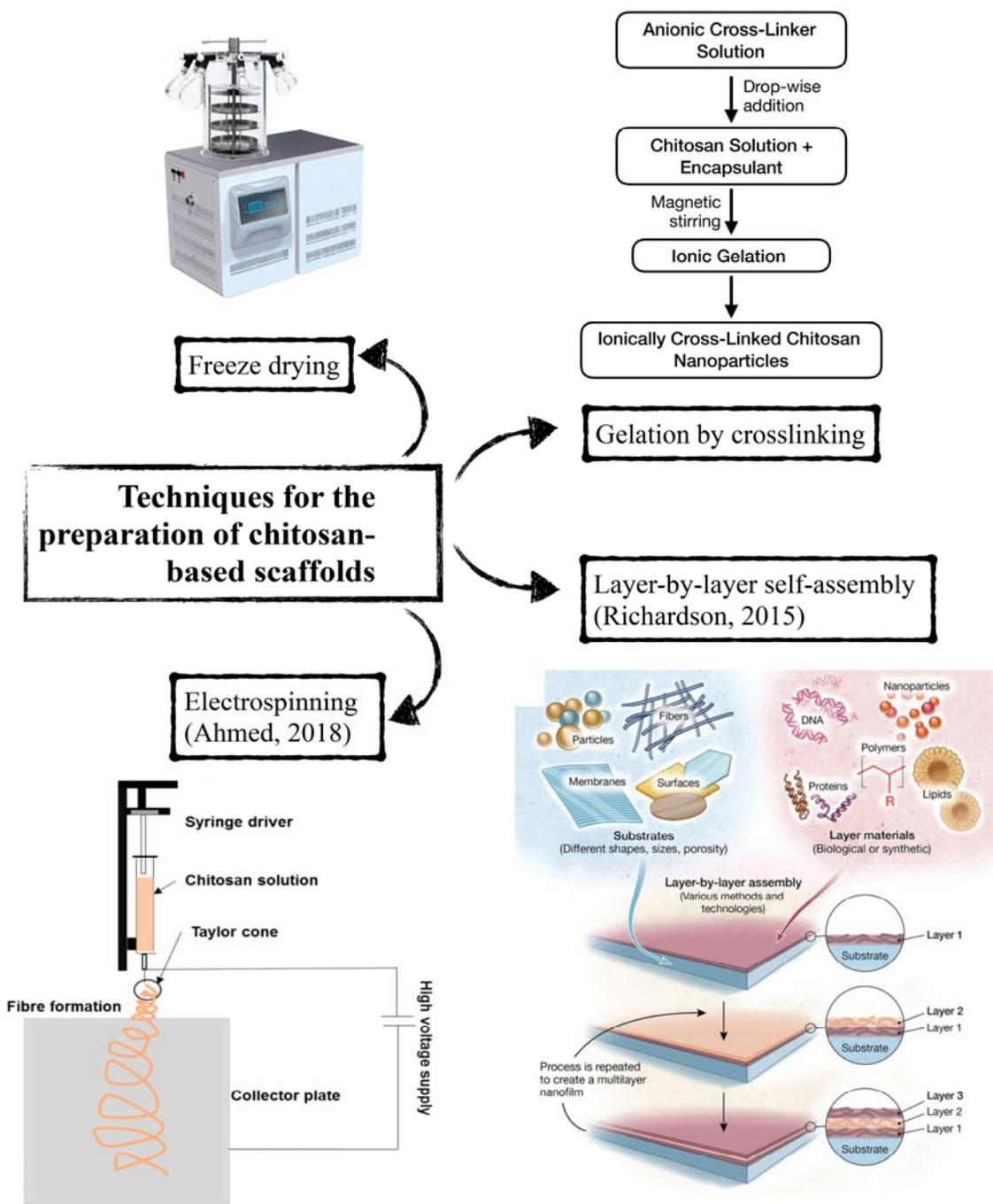
**Figure 3.** Techniques for the preparation of chitosan-based scaffolds. Adapted with permission from Refs. [61,72]. [61], Copyright 2018, Elsevier. [72], Copyright 2015, Science.
