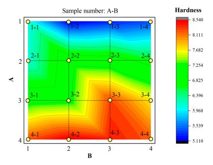
Figure 6. Trends in the indentation hardness of Ti-Zr-Nb-Ta alloys.
