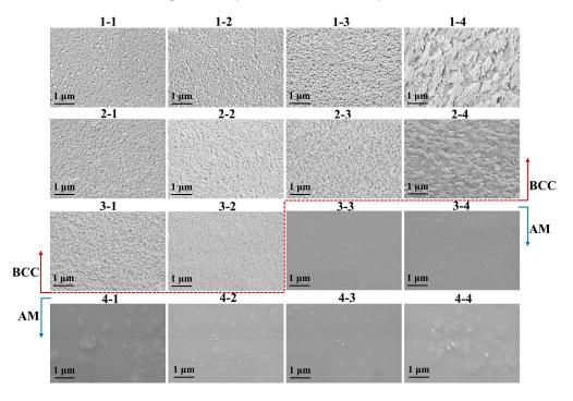
Figure 5. SEM images of the deposited Ti-Zr-Nb-Ta alloys taken from the surface.
