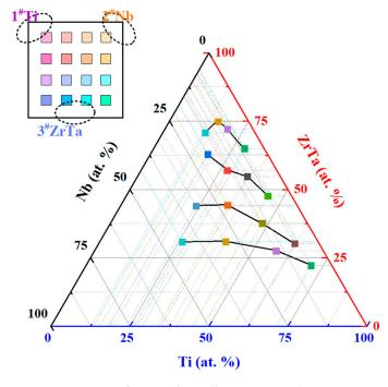
Figure 2. Location of Ti-Zr-Nb-Ta alloys in a pseudo-ternary compositional map.
