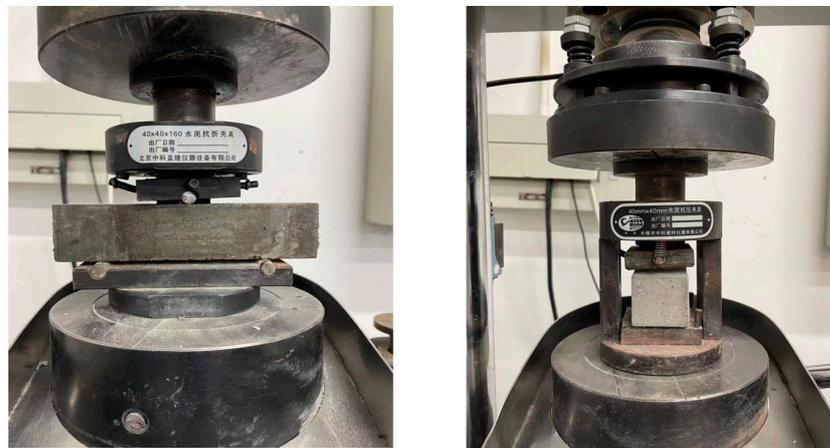
**The measurement of flexural strength**    **The measurement of compressive strength**
