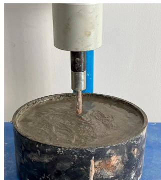
**Figure 2.** The measurement of initial setting time.
