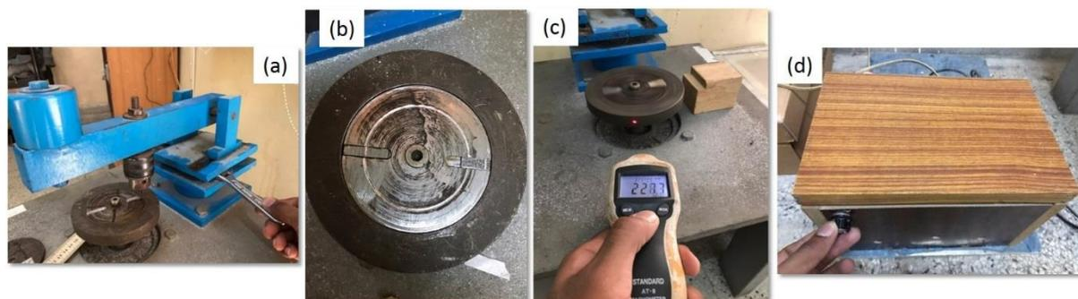
**Figure 3.** Execution sequence of wear testing; (a) wear testing machine, (b) fixture having two slots placed onto the disc holder is separately (c) tachometer, (d) controller box.
