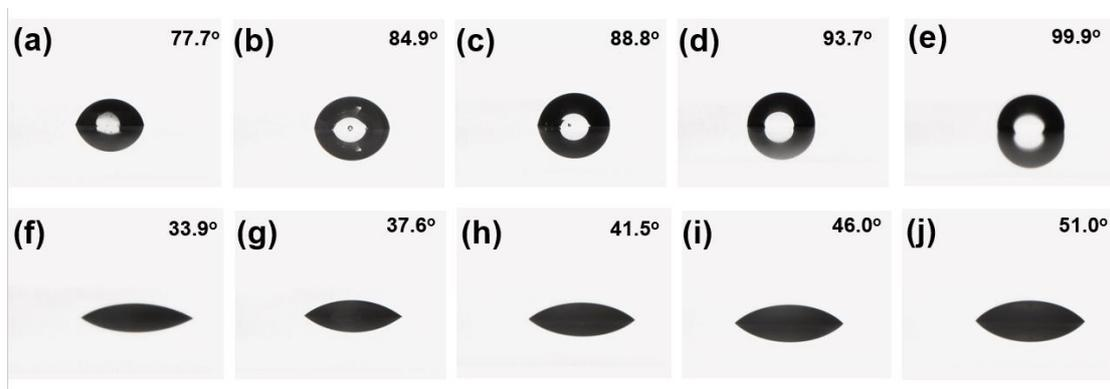
**Figure 12.** Water and cetane contact angle of fluorocarbon polyurethane amino baking paint films after abrasion of the paint films with a microprocessor: (a) water on F3; (b) water on F6; (c) water on F7; (d) water on F8; (e) water on F9; (f) cetane on F3; (g) cetane on F6; (h) cetane on F7; (i) cetane on F8; (j) cetane on F9.
