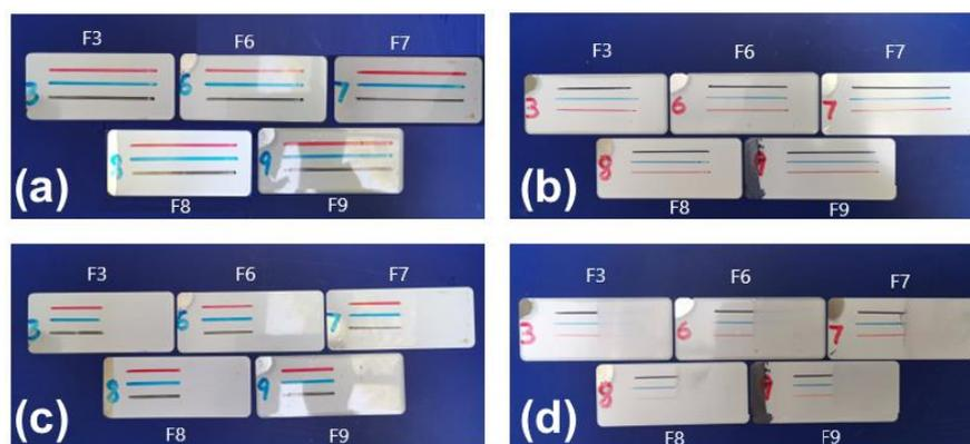
**Figure 14.** Fluorocarbon polyurethane amino baking paint film graffiti resistance test: (a) red, blue, and black alcohol-soluble whiteboard marker markings on F3 and F6–F9; (b) red, blue, and black oily marker markings on F3 and F6–F9; (c) half lines of (a) erased 24 h later; (d) half lines of (b) erased 24 h later.
