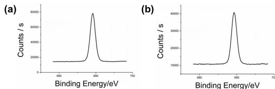
Figure 8. XPS comparison of fluorine content on the surface of fluorocarbon polyurethane baking paint: (a) F3 XPS pattern of fluorine content of the surface of formulation; (b) F4 XPS pattern of fluorine content of the surface.
