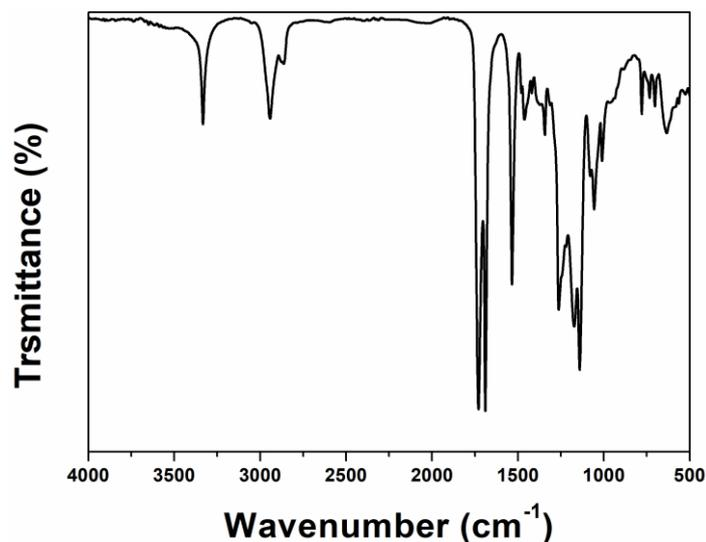
Figure 5. Infrared spectrum of Resin-FPU-OH.
