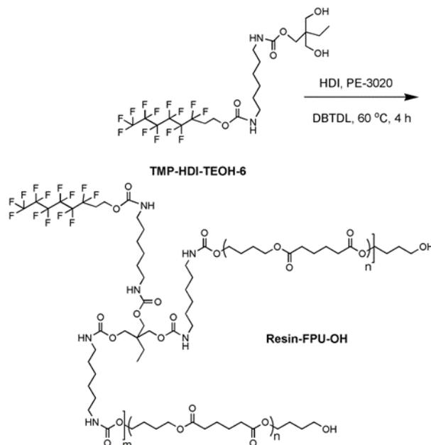
**Figure 2.** Synthesis of fluorocarbon polyurethane hydroxy resins.
