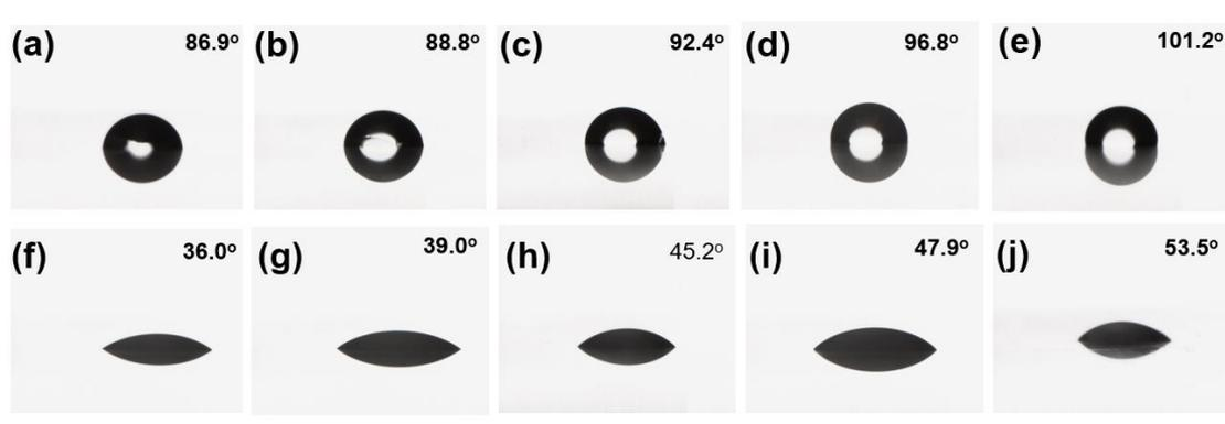
**Figure 13.** Water and cetane contact angles of fluorocarbon polyurethane baking paint films after alcohol wipes: (a) water on F3; (b) water on F6; (c) water on F7; (d) water on F8; (e) water on F9; (f) cetane on F3; (g) cetane on F6; (h) cetane on F7; (i) cetane on F8; (j) cetane on F9.
