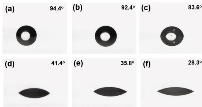
**Figure 9.** Fluorocarbon polyurethane amino baking paint film water and cetane contact angles: (a) water on F3; (b) water on F4; (c) water on F5; (d) cetane on F3; (e) cetane on F4; (f) cetane on F5.
