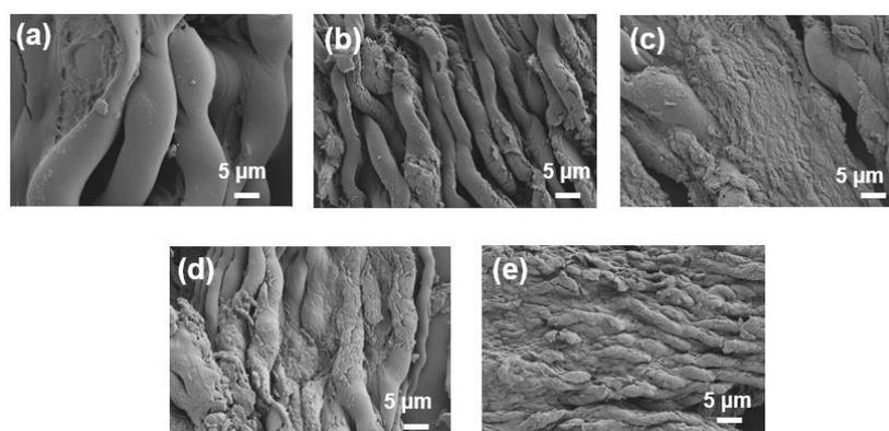
**Figure 11.** SEM photos of fluorocarbon polyurethane baking paint film: (a) F3 SEM photo; (b) F6 SEM photo; (c) F7 SEM photo; (d) F8 SEM photo; (e) F9 SEM photo.
