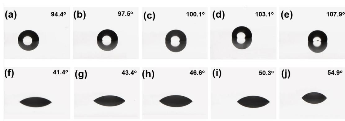
**Figure 10.** Initial water and cetane contact angles of fluorocarbon polyurethane baking paint: (a) water on F3; (b) water on F6; (c) water on F7; (d) water on F8; (e) water on F9; (f) cetane on F3; (g) cetane on F6; (h) cetane on F7; (i) cetane on F8; (j) cetane on F9.
