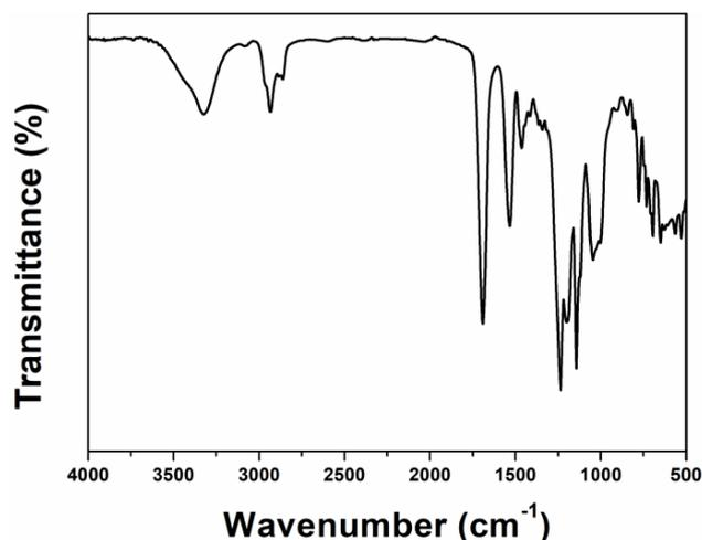
Figure 3. Infrared spectra of TMP-HDI-TEOH6.
