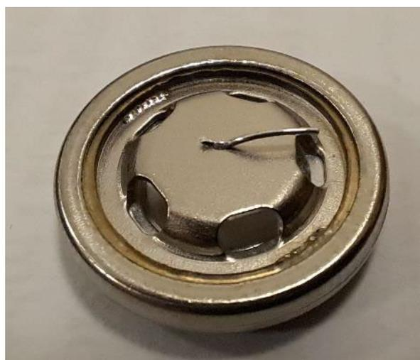
**Figure 1.** Wire bond visible on battery cap after cutting off top of battery cell.
