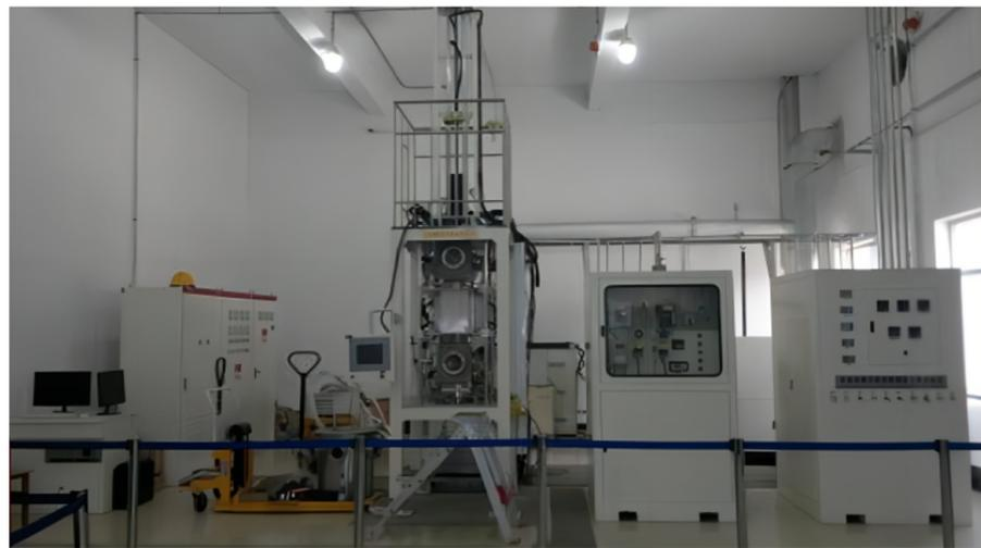
**Figure 5.** CGA-2010 multi-functional galvanizing process simulation equipment.
