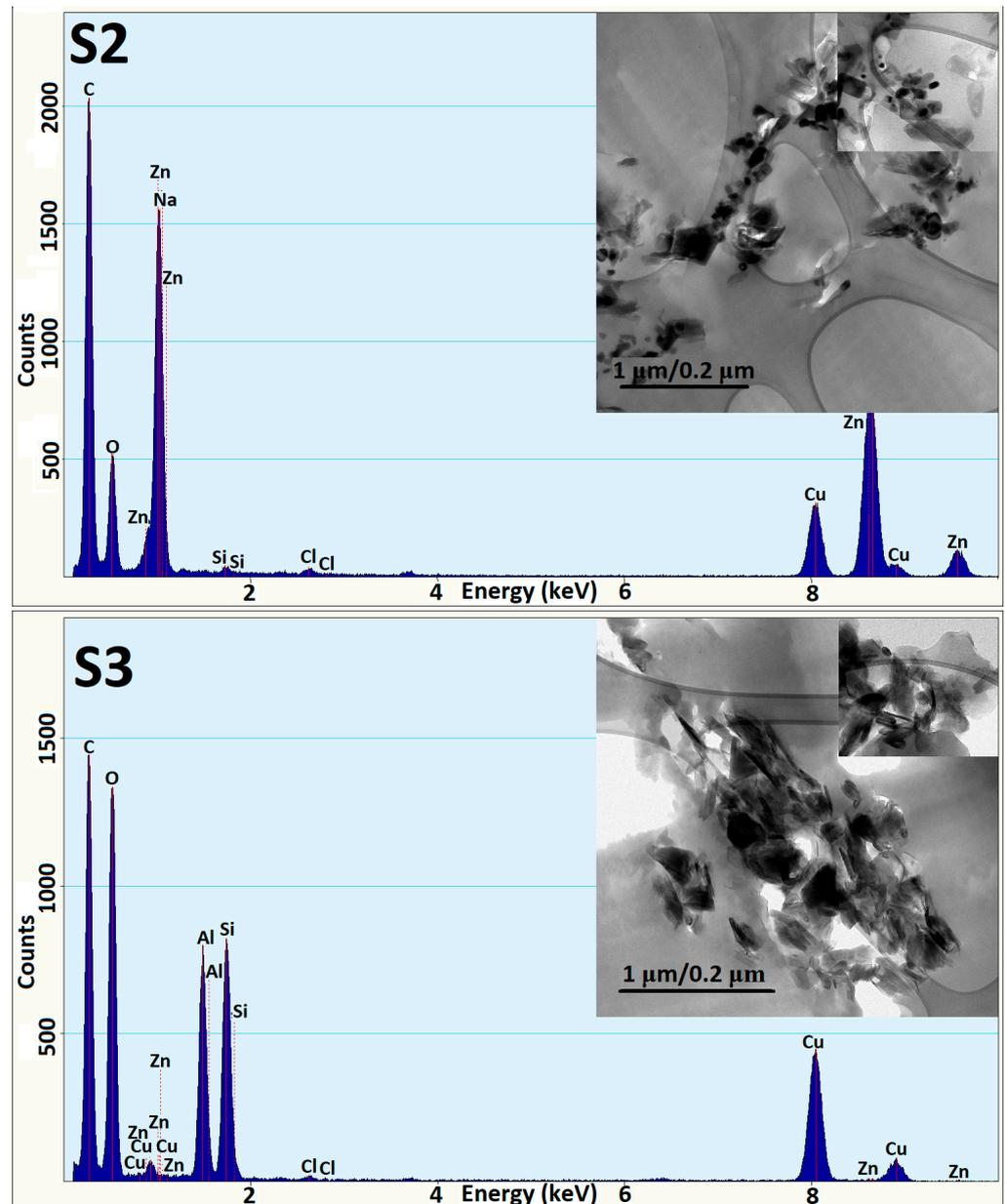
Figure 6. TEM images and EDX analysis of samples S1–S3.
