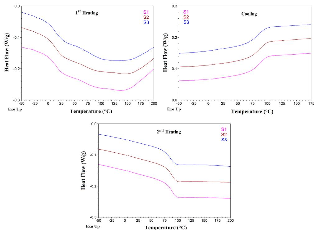
**Figure 5.** DSC curves of samples (top—first heating; down—second heating) S1–S3.
