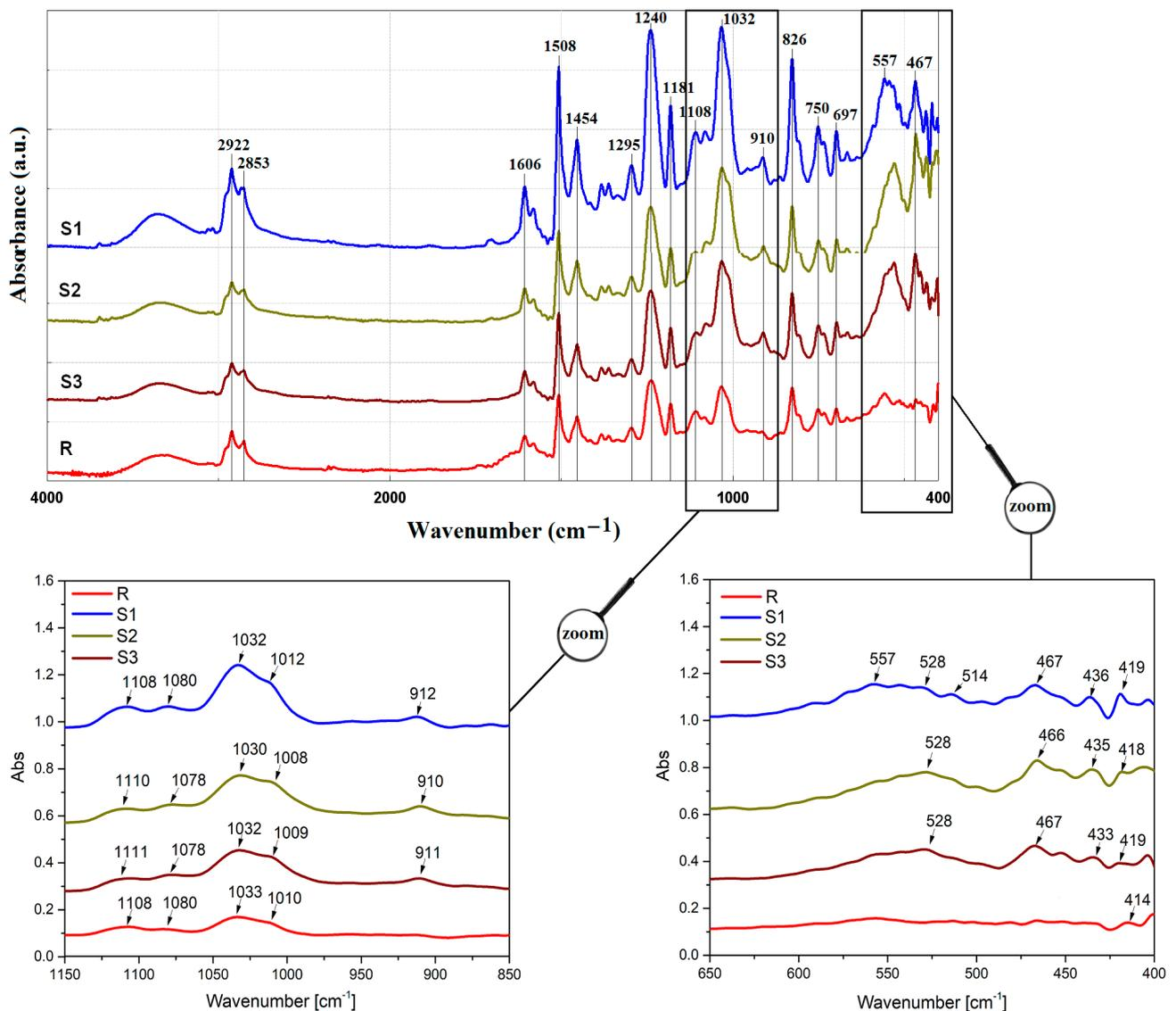
**Figure 3.** FTIR-ATR spectra of samples S1–S3 and of epoxy resin (R).
