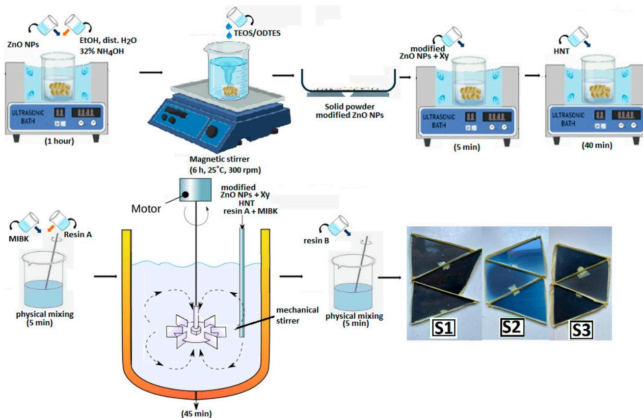
**Figure 1.** Schematic illustration of synthesis procedure to obtain modified ZnO/epoxy resin composites.
