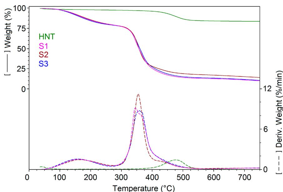
**Figure 4.** Thermogravimetric analysis curves of samples: HNT, S1, S2, S3 and S4.
