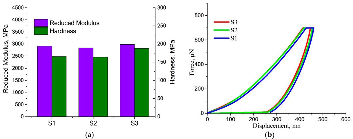
**Figure 7.** (a) Indentation reduced modulus and hardness; (b) force vs. displacement curves of samples S1–S3.
