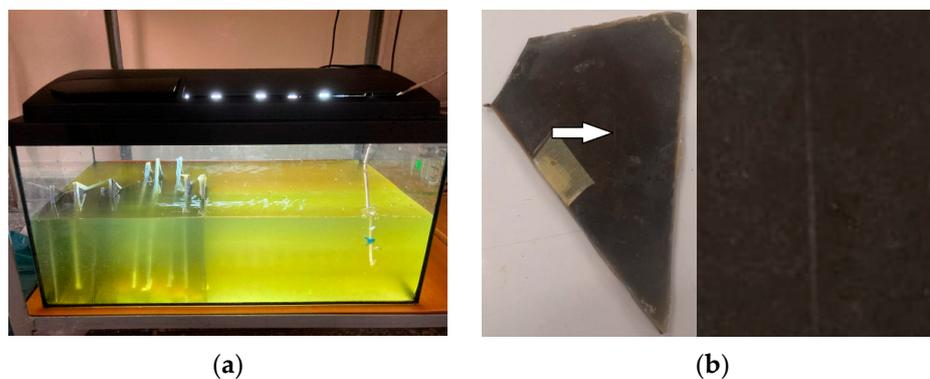
**Figure 9.** (a) Metal surfaces coated with samples and kept in seawater; (b) sample S3 after scratching test (the scratch is pointed by the white arrow).
