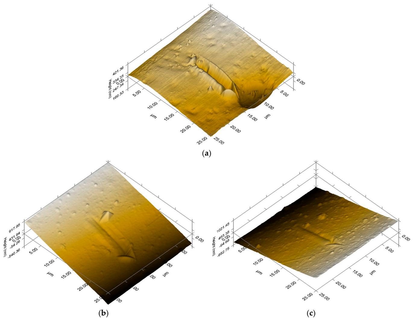
**Figure 8.** Three-dimensional plot of SPM image after scratching for samples: (a) S1; (b) S2; (c) S3.
