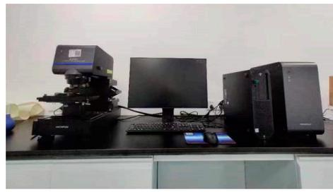
Figure 9. Confocal Laser Scanning Microscope.
