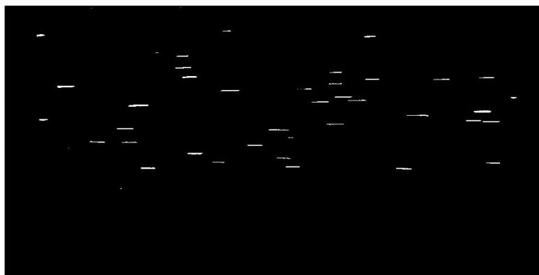
**Figure 11.** Figure 10 cropped and analyzed for particle velocities. A yellow streak was placed over the length of each particle streak the program identified.
