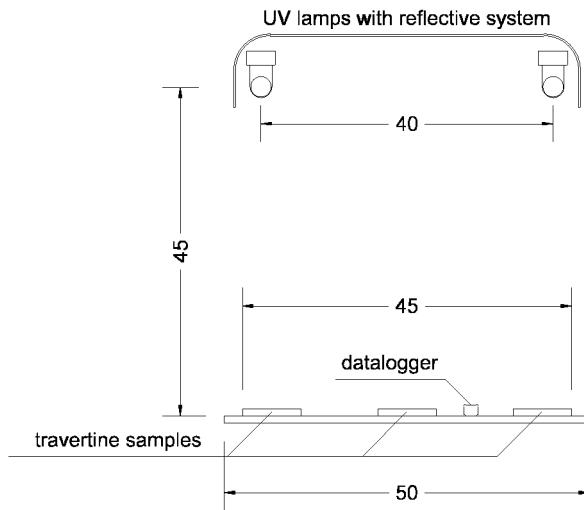
**Figure 1.** Diagram of the laboratory system used to perform the self-cleaning test.
