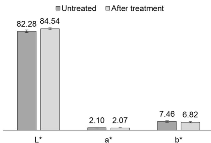
**Figure 3.** Average chromatic values according to CIELAB system before and after  $TiO_2$  treatment.
