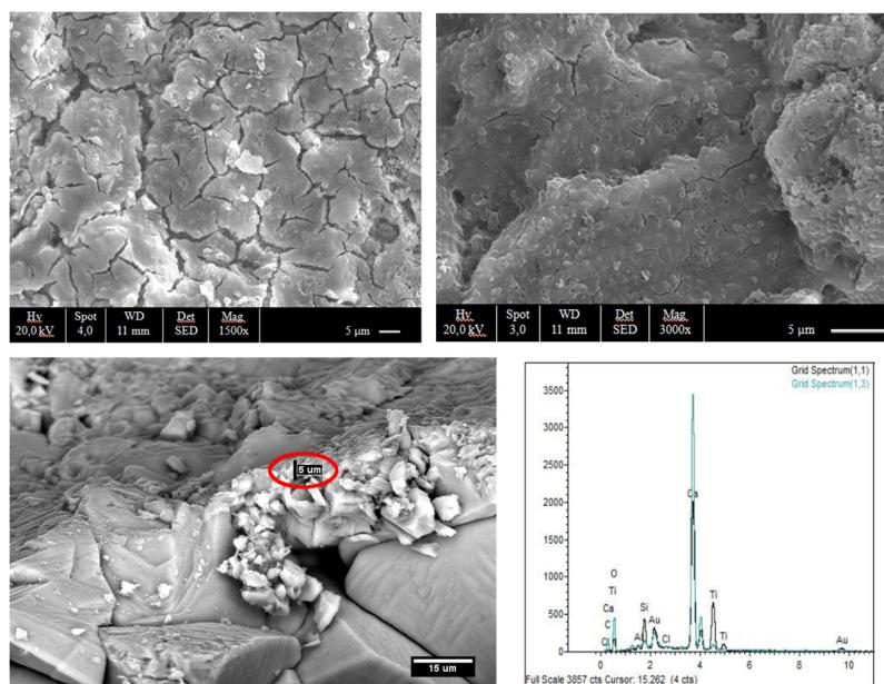
**Figure 2.** Scanning electron microscopy/energy dispersive X-ray spectroscopy (SEM/EDX) analysis of treated samples: surface morphology (SED, magnitude 1500× and 3000×); cross-section (BSD, titanium is colored bright white) with a reference scale for measuring the thickness of the coating and EDX spectra (two different measurement points). Details about the parameters (voltage, spot size, working distance) set during the analysis are also reported.
