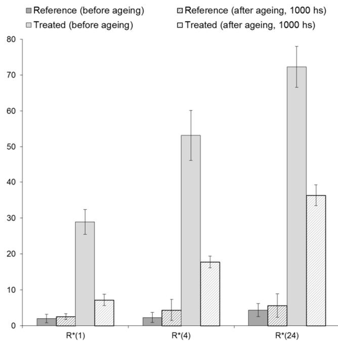
**Figure 4.** Average values of the parameter  $R_E^*$  describing the intensity of self-cleaning efficiency during test procedure (after 1, 4 and 24 h of exposure to UV light) on treated and untreated surfaces. The results refer to the performances measured at time zero (before ageing) and at the end of the 1000 h-long weathering procedure (after ageing).
