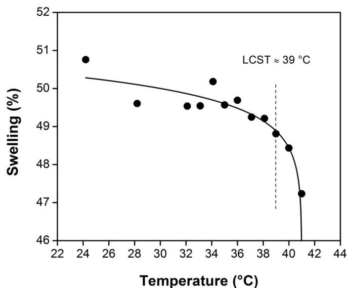
**Figure 7.** Temperature dependence of the swelling ratio in water as a function of temperature for poly(NVCL-co-NVIM)-grafted SR film (90% graft).
