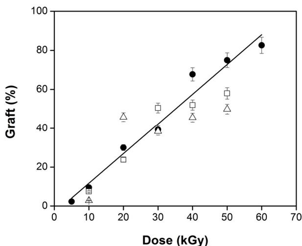
**Figure 2.** Grafting yield by one step method of PNVCL and PNVIM onto SR films in toluene as function of irradiation dose, at dose rate of 9.3 kGy h<sup>-1</sup> and different monomer concentration: 50% monomer in toluene (NVCL/NVIM 1/1, vol%) (●); 50% monomer in toluene (NVCL/NVIM 7/3, vol%) (□); and 100% monomer (NVCL/NVIM 1/1, vol%) (△).
