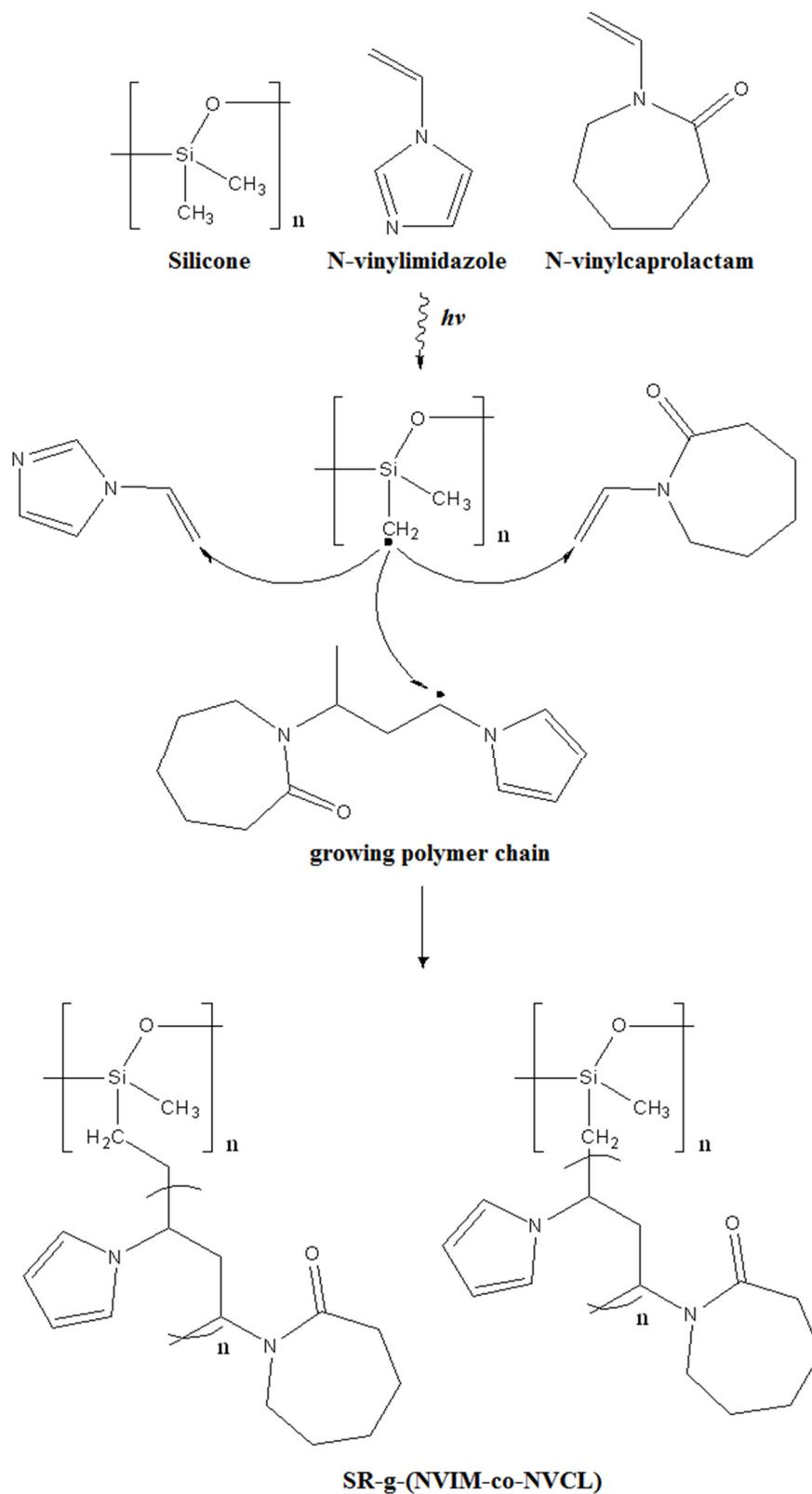
**Scheme 1.** Grafting of SR-g-(NVCL-co-NVIM) by means of gamma radiation.
