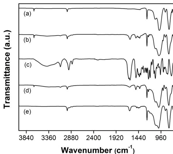
**Figure 4.** FTIR-ATR spectra for SR (a), SR-g-(NVCL-co-NVIM) 75% graft (b), poly(NVCL-co-NVIM) (c), SR-g-NVIM 106% graft (d), and SR-g-NVCL 29% graft (e).
