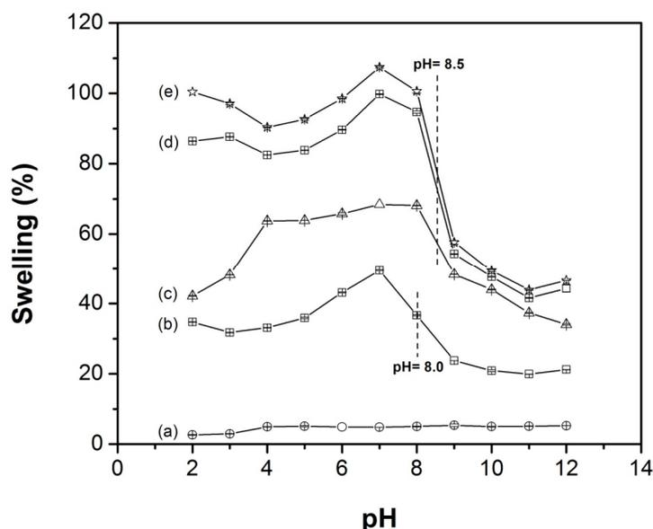
**Figure 9.** Dependence of swelling degree with respect to pH for SR-g-(NVCL-co-NVIM) at different grafting yield: 7.5% graft (a), 24% graft (b), 50% graft (c), 52% graft (d), and 59% graft (e).
