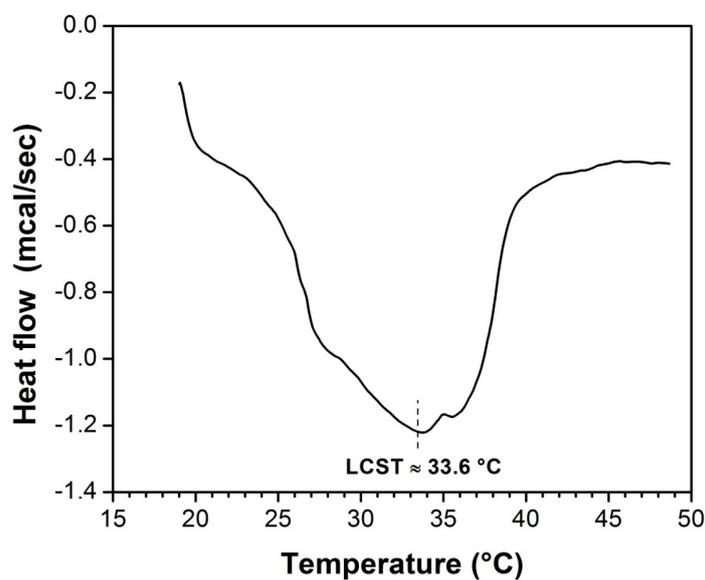
**Figure 8.** DSC thermograms of swelled SR-g-(NVCL-co-NVIM) with distilled water at a heating rate of  $1\text{ °C min}^{-1}$  from 20 to 50 °C. LCST is indicated.
