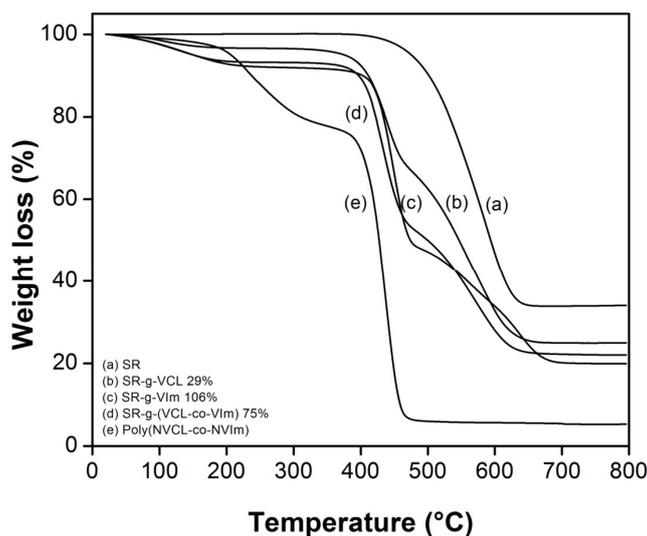
**Figure 5.** Thermogravimetric curves for SR alone (a), SR-g-VCL 29% graft (b), SR-g-VIM 106% graft (c), SR-g-(VCL-co-VIM) 75% (d), and poly(NVCL-co-NVIM) (e).
