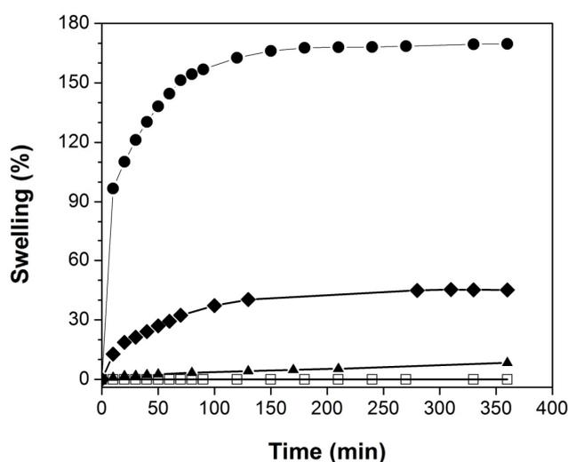
**Figure 3.** Swelling kinetics of PNVCL and PNVIM onto SR films graft contents of SR alone (□), SR-g-NVCL 29% graft (▲), SR-g-(NVCL-co-NVIM) 75% graft (◆), and SR-g-NVIM 106% graft (●) immersed in water at 25 °C.
