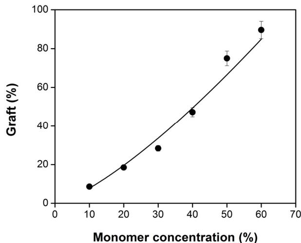
**Figure 1.** Grafting yield by one step method of poly(N-vinylcaprolactam) (PNVCL) and poly-(N-vinylimidazole) (PNVIM) onto silicone rubber (SR) films as function of monomer concentration in toluene, dose fixed of 50 kGy and dose rate of 9.3 kGy h<sup>-1</sup>.
