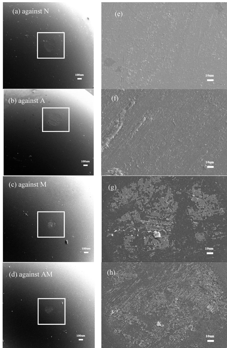
**Figure 8.** The SEM images of the counterface balls ( $\text{Si}_3\text{N}_4$  ball) after sliding against (a) A, (b) B, (c) C, and (d) D and corresponding higher magnification SEM images against (e) A, (f) B, (g) C, and (h) D.
