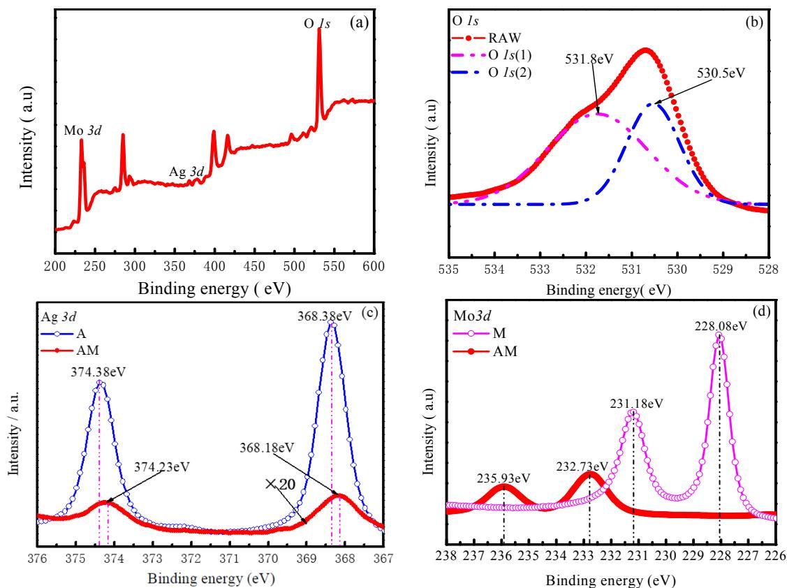
**Figure 3.** (a) XPS full spectra; (b) O<sub>1s</sub> XPS spectra for AM; (c) Ag<sub>3d</sub> XPS spectra of A and AM; and (d) Mo<sub>3d</sub> XPS spectra of M and AM before the wear test.
