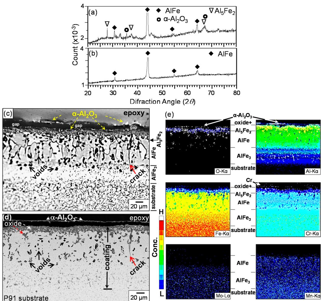
**Figure 5.** Al hot-dipped P91 steel after oxidation at 800 °C for 100 h. (a) XRD pattern before grinding; (b) XRD pattern after grinding off the surface; (c) cross-sectional optical microstructure (etched); (d) EPMA BSE cross-sectional image; (e) EPMA maps of (d).
