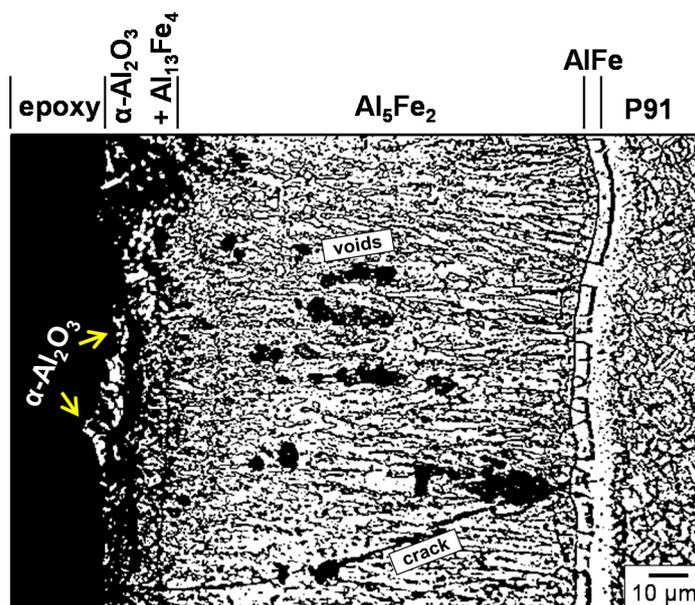
**Figure 4.** Optical microstructure of Al hot-dipped P91 steel after oxidation at 700 °C for 100 h (etched).
