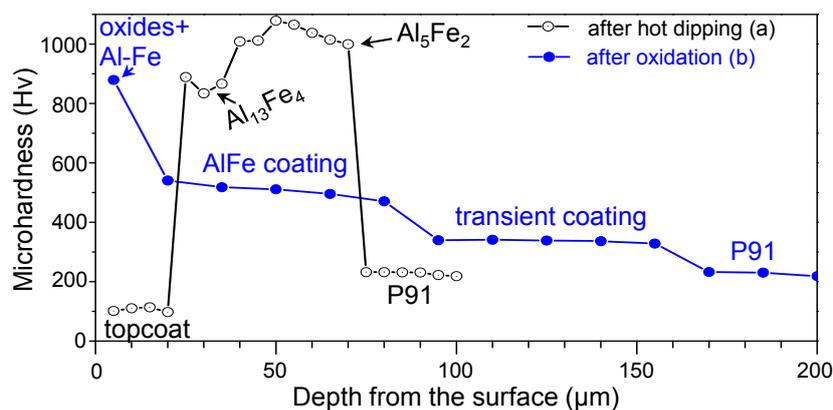
**Figure 6.** Vickers microhardness variation along the depth for Al-hot dipped P91 steel: (a) before oxidation; (b) after oxidation at 800 °C for 100 h.
