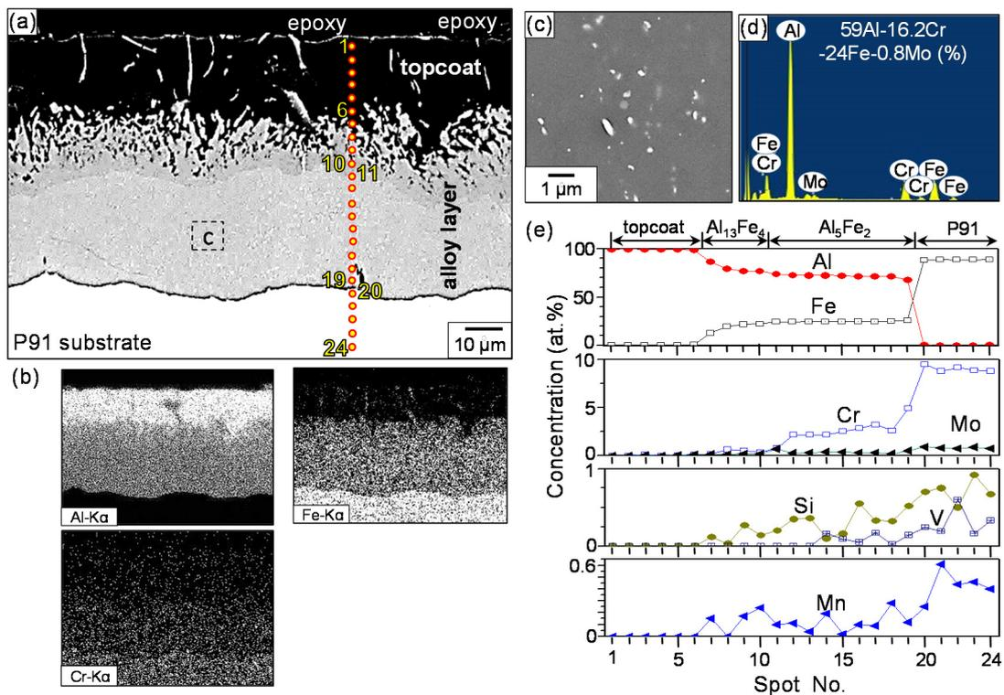
**Figure 2.** Al hot-dipped P91 steel. (a) SEM cross-sectional back-scattered electron (BSE) image (etched); (b) EDS maps of (a); (c) enlarged image of the rectangular area marked in (a); (d) EDS spectrum of white particles shown in (c); (e) EDS concentration profiles along the spots 1–24 marked in (a).
