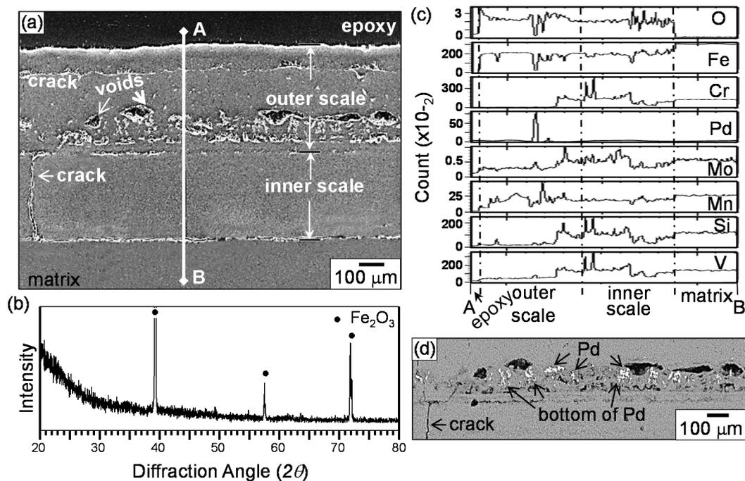
**Figure 8.** Uncoated P91 steel after oxidation at 900 °C for 20 h: (a) cross-sectional EPMA image (unetched); (b) XRD pattern; (c) EPMA line profiles along A–B marked in (a); (d) enlarged SEM-BSE image around the outer/inner oxide scale shown in (a).
