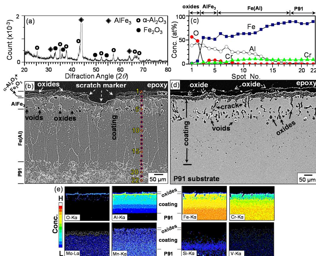
**Figure 7.** Al hot-dipped P91 steel after oxidation at 900 °C for 20 h: (a) XRD pattern; (b) cross-sectional SEM image (etched); (c) EDS concentration profiles along spots 1–22 marked in (b); (d) cross-sectional EPMA image (unetched); (e) EPMA maps of (d).
