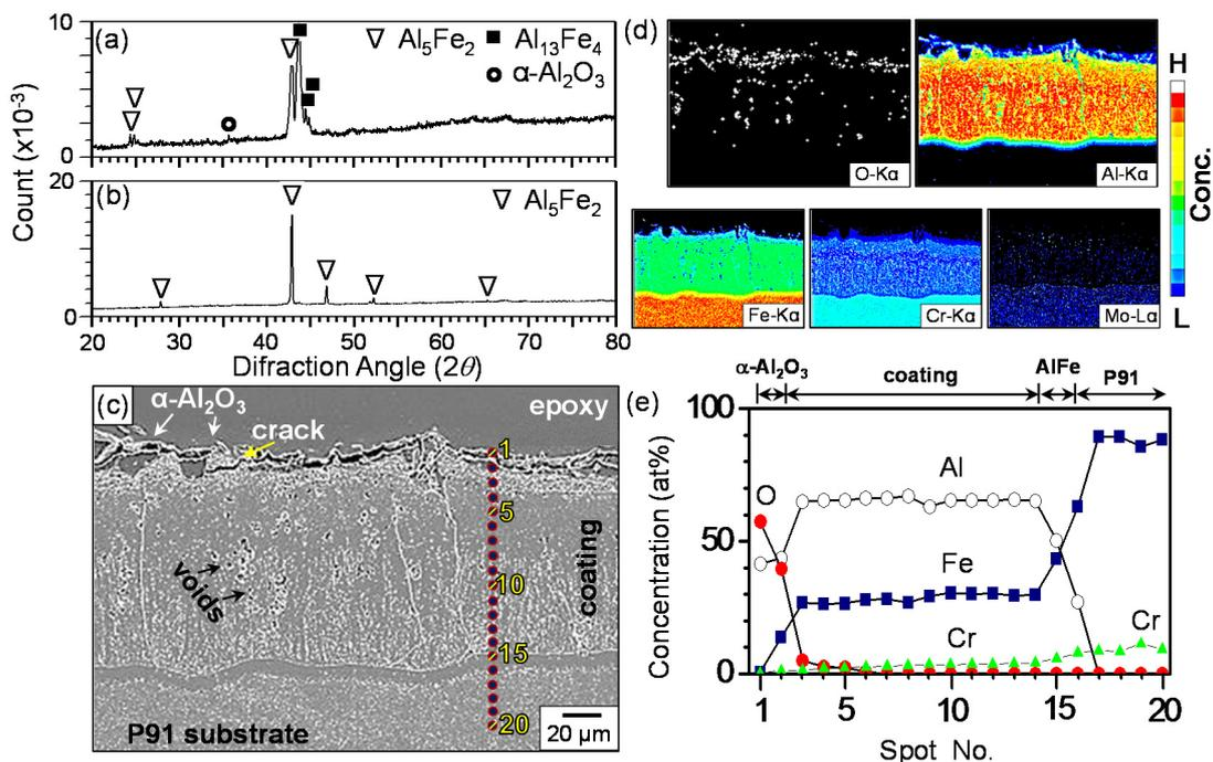
**Figure 3.** Al hot-dipped P91 steel after oxidation at 700 °C for 100 h. (a) XRD pattern before grinding; (b) XRD pattern after grinding off the surface; (c) etched electron probe microanalyzer (EPMA) cross-sectional image; (d) EPMA maps of (c); (e) EDS concentration profiles along spots 1–20 marked in (c).
