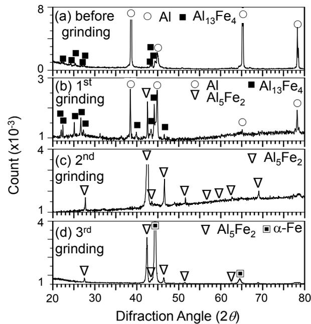
**Figure 1.** XRD patterns of the Al hot-dipped P91 steel: (a) before grinding; (b) after first grinding; (c) after second grinding; (d) after third grinding.
