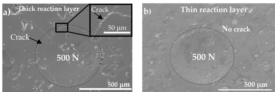
**Figure 4.** SEM images showing the impressions of ball indentations on the surface of thick after applying a load of 500 N (a), and thin reaction layers after applying a load of 500 N (b). Reproduced from [101] with permission from Elsevier.
