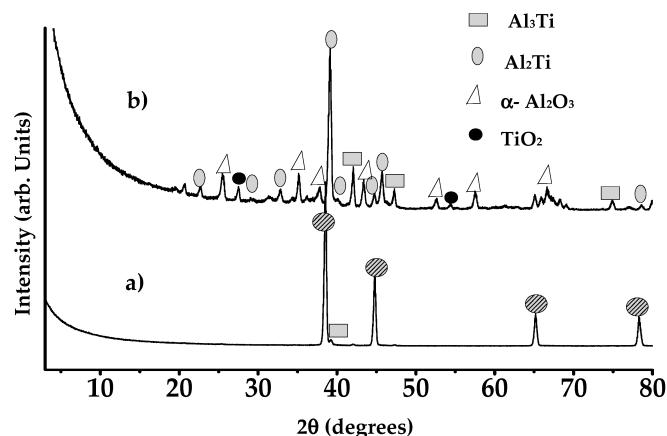
**Figure 5.** TF-XRD of Al layer on the Ti alloy after heat treatment at 640 °C for 12 h (**a**) and subsequent heat treatment at 850 °C for 96 h (**b**) both in an air atmosphere. Reproduced from [100] with permission from Trans Tech.
