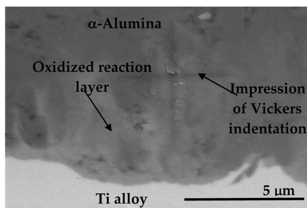
**Figure 10.** BSE image show sectional view of alumina layer-reaction layer-Ti alloy and impression of Vickers indentation at alumina-Ti interface. Reproduced from [102] with permission from Elsevier.
