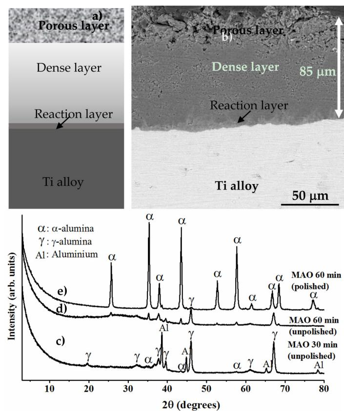
**Figure 7.** Schematic view of section of designed alumina/Ti alloy model (a); corresponding BSE image of alumina layer on the Ti alloy (b); and TF-XRDs of CS-Al layer after MAO for 30 min (c); 60 min (d); and after polishing (e). Reproduced from [101] with permission from Elsevier.
