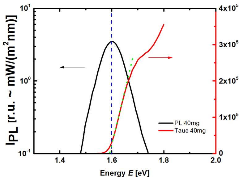
**Figure S3.** Tauc gap from SPV and PL spectrum for 40mg/mL of PMMA.
