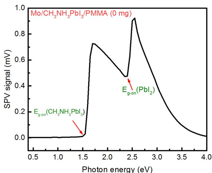
**Figure S1.** SPV spectra of perovskite on molybdenum substrate coated with 0 mg of PMMA in in 1 mL of butyl acetate.
