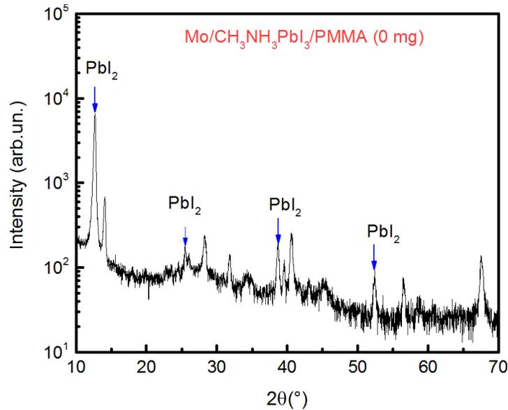
**Figure S2.** Grazing incidence X-ray diffraction (GIXRD) pattern for of  $\text{CH}_3\text{NH}_3\text{PbI}_3$  on molybdenum substrate coated with 0 mg of PMMA in 1 ml of butyl acetate after storage in air for 50 days.
