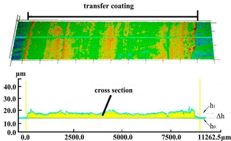
Figure 2. Measuring principle of the transfer layer thickness.
