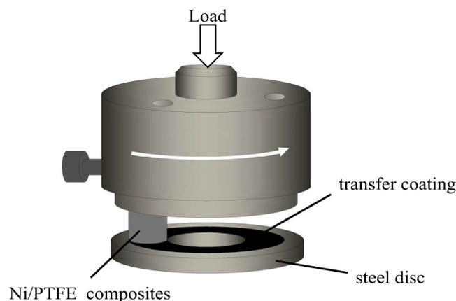
**Figure 1.** Schematic diagram of the pin-on-disc tribometer.
