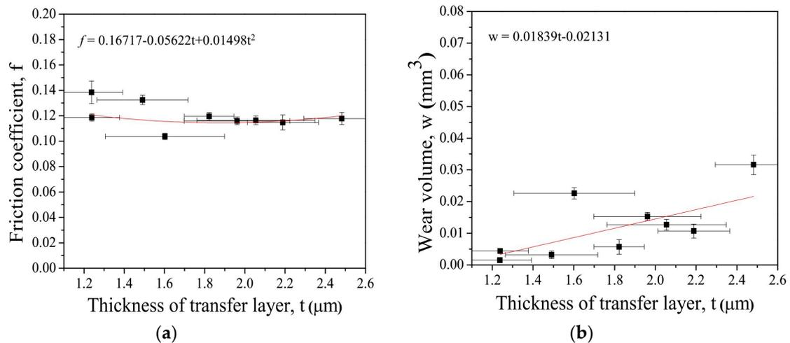
**Figure 11.** Relationships between tribological properties and transfer layer thickness: (a) Friction coefficient, (b) wear volume.
