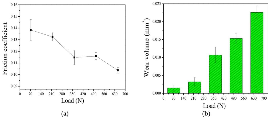
**Figure 7.** The change of friction coefficient and wear under different loads: (a) Friction coefficient vs. load; (b) wear volume vs. load.
