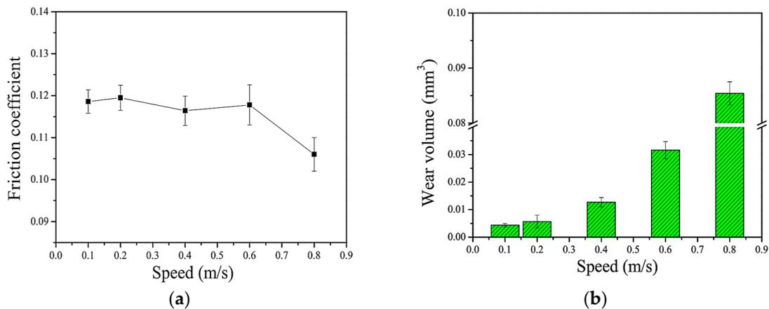
**Figure 3.** The change of friction coefficient and wear under different speeds: (a) Friction coefficient vs. speed; (b) wear volume vs. speed.
