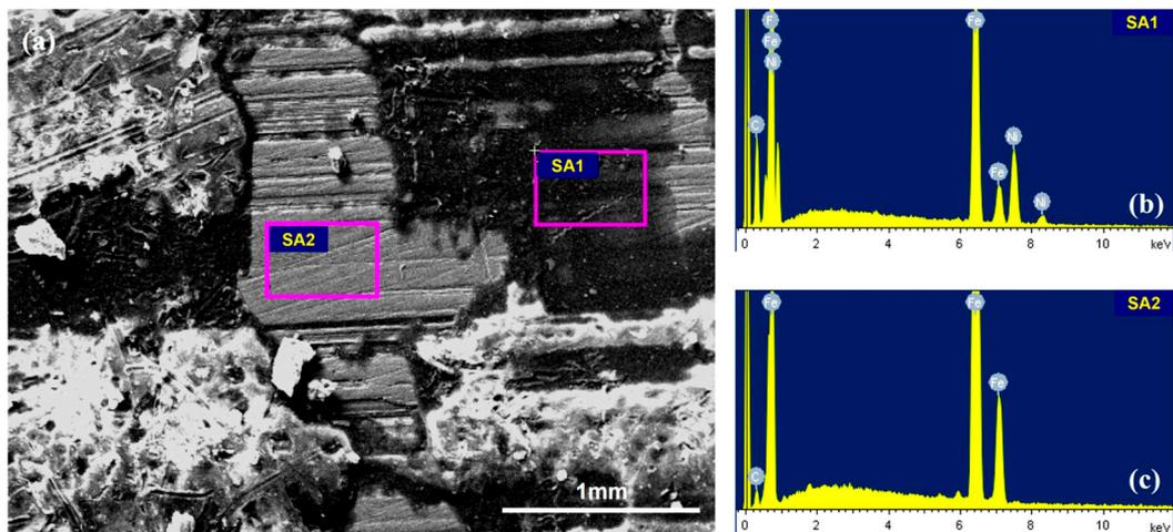
**Figure 5.** SEM and EDS images of the steel surface with and without transfer layers: (a) Steel surface with the discontinuous transfer layer; (b) EDS image of area SA1; (c) EDS image of area SA2.
