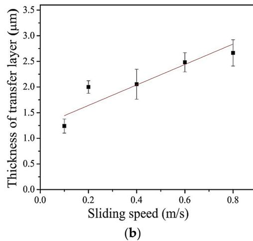
**Figure 6.** (a) The height distribution mappings of transfer layers formed under different sliding speeds; (b) The average transfer layer thickness vs. sliding speed.
