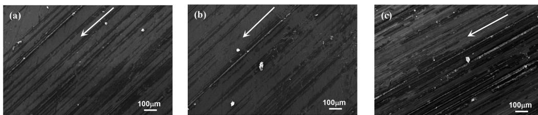
**Figure 8.** SEM images of the transfer layers under different loads: (a) 72 N; (b) 362 N; (c) 651 N.
