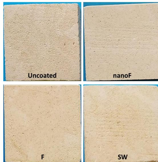
Figure 5. Uncoated and coated PS stone surfaces.
