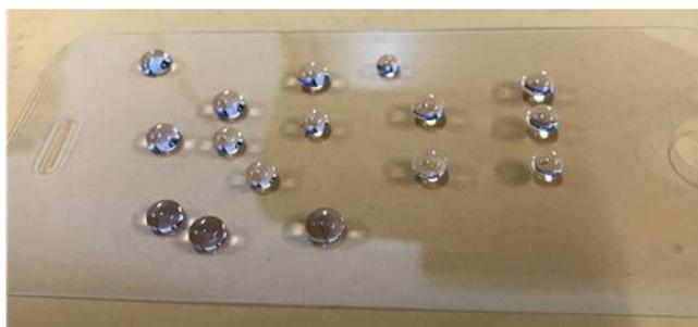
Figure 9. Hydrophobicity of FSi@SiO<sub>2</sub> coating on mobile phone screen.
