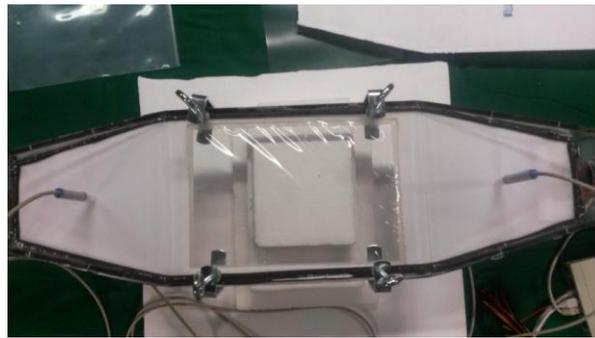
**Figure 2.** Support including the membrane for the base unit (plate) of the enthalpy heat exchanger.
