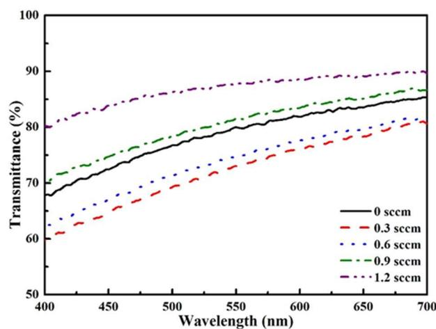
**Figure 5.** The transmittance spectra of SiO<sub>x</sub>:DLC films with the different HMDSO flow rates. (RF bias = 400 V, DC power = 50 W, CH<sub>4</sub> = 12.5 sccm, thickness = 65 ± 5 nm).
