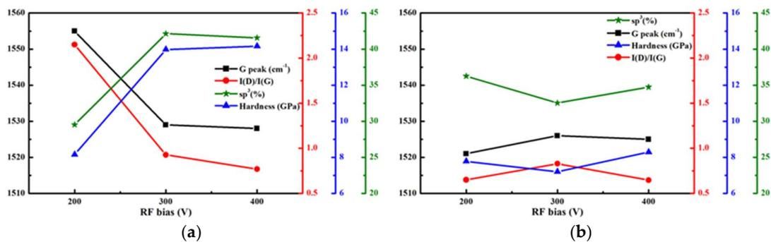
**Figure 2.** The analysis of DLC properties in the RF bias range of 200–400 V (a) with, and (b) without DC power of 50 W with  $\text{CH}_4$  flow rate of 15 sccm. ( $\text{CH}_4 = 15$  sccm, thickness: (a) 470 nm and (b) 110 nm).
