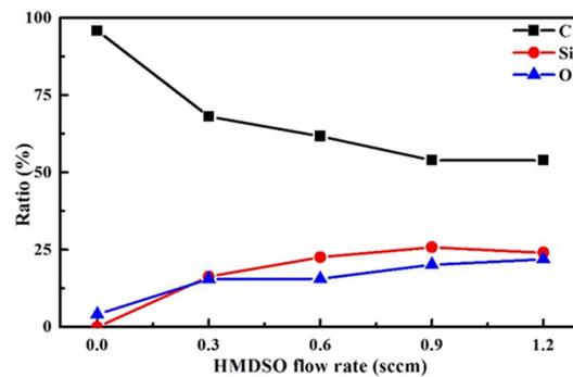
**Figure 7.** The X-ray photoelectron spectroscopy (XPS) relative atomic content of C, Si, and O at the different HMDSO flow rates. (RF bias = 400 V, DC power = 50 W, CH<sub>4</sub> = 12.5 sccm, thickness = 65 ± 5 nm).
