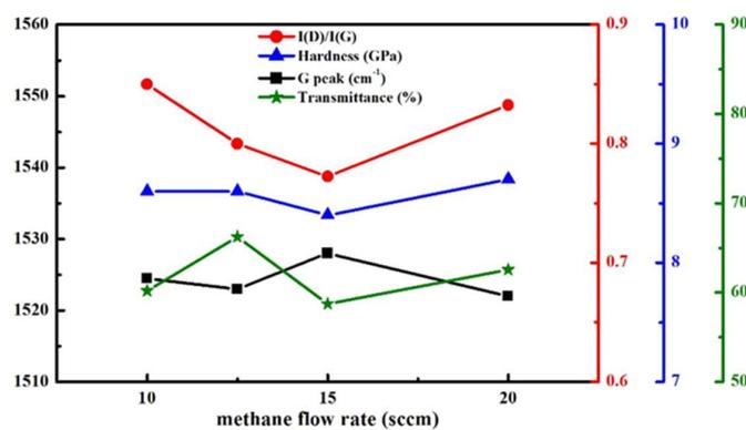
**Figure 4.** The analysis of DLC properties and transmittance at the different  $\text{CH}_4$  flow rates with RF bias of 400 V and DC power of 50 W. (thickness =  $135 \pm 10$  nm).
