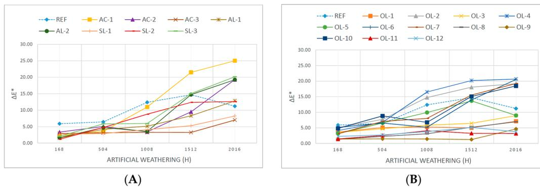
**Figure 4.** The total colour difference of acrylate, alkyd, synthetic (A) and oil-based (B) coating systems applied to Siberian larch during artificial weathering lasting 168, 504, 1512 and 2016 h.
