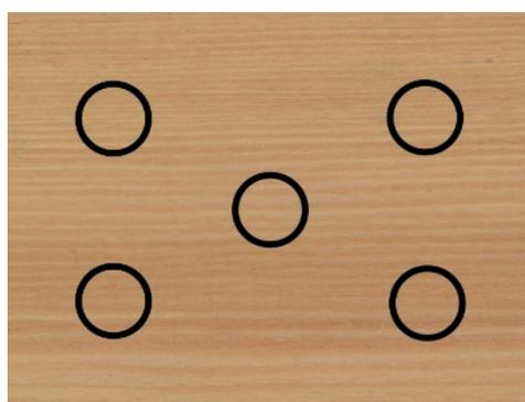
**Figure 2.** Template used to ensure that locations of colour measurements on samples was the same at each exposure interval—measuring area was given using  $d/8$  mm geometry of spectrophotometer.
