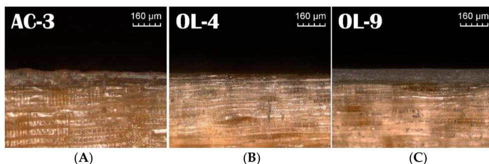
**Figure 1.** Images from confocal laser scanning microscope showing a typical film of thick acrylate coating ((A) AC-3 in this case), penetrating oils ((B) OL-4 in this case) and oil-based coatings also creating a surface layer ((C) OL-9 in this case) after application. It is possible to see only very poor penetration into the first layer of tracheids in the impermeable larch heartwood.
