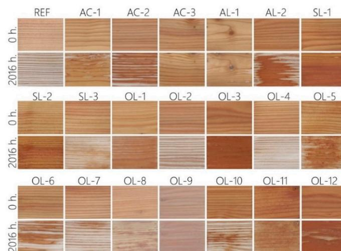
**Figure 6.** Visual evaluation of coating systems applied to European larch before (0 h) and after (2016 h) AW.
