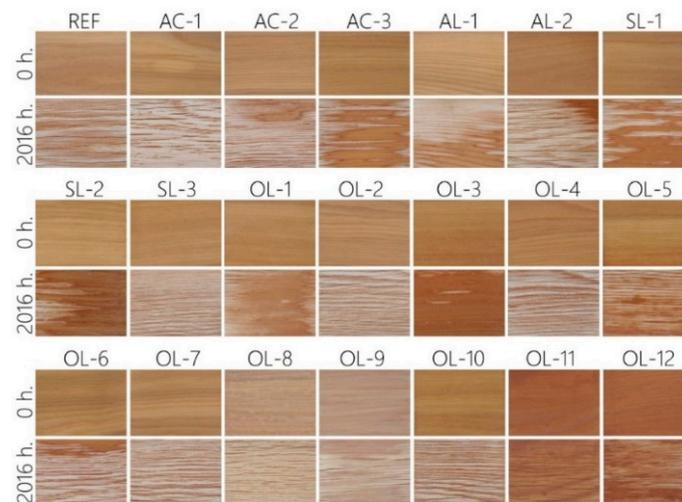
**Figure 7.** Visual evaluation of coating systems applied to Siberian larch before (0 h) and after (2016 h) AW.
