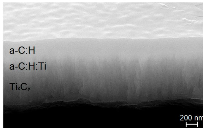
**Figure 3.** SEM image of cross section of the underlying Ti/Ti<sub>x</sub>C<sub>y</sub>/a-C:H:Ti/a-C:H layer system (perspective view).
