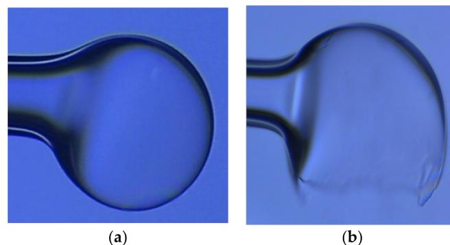
**Figure 3.** Failed experiment and the specific reason. (a) Deformation due to the gravity; (b) deformation due to non-uniform wall thickness.
