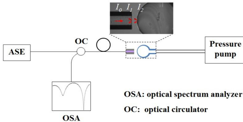
**Figure 5.** Experimental setup for measuring the pressure sensitivity of the fabricated single-ended microbubble.
