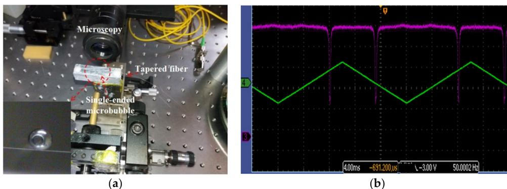
Figure 9. Experimental system and the output WGM spectrum. (a) Experimental setup of the WGM system; (b) screen shot of the output spectrum.
