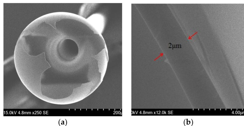
**Figure 4.** Result of SEM experiment. (a) Collapsed single-ended microbubble; (b) measured wall thickness.
