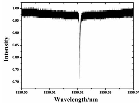
**Figure 10.** Output spectrum of the proposed single-ended microbubble-based WGM resonator.
