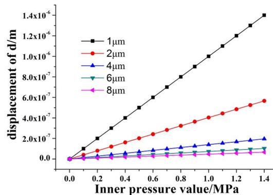
Figure 12. Relationship of bubble tip shift and inner pressure under different wall thickness (from 1 to 8  $\mu\text{m}$ ).
