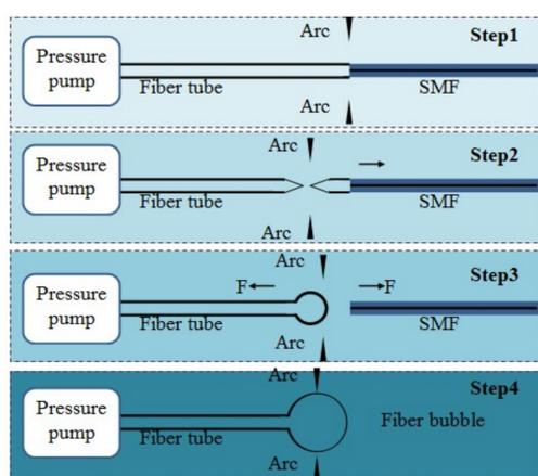
**Figure 1.** Fabrication processes of the proposed single-ended microbubble.
