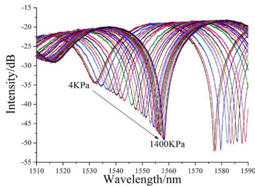
**Figure 6.** FP interference spectrum of the microbubbles.
