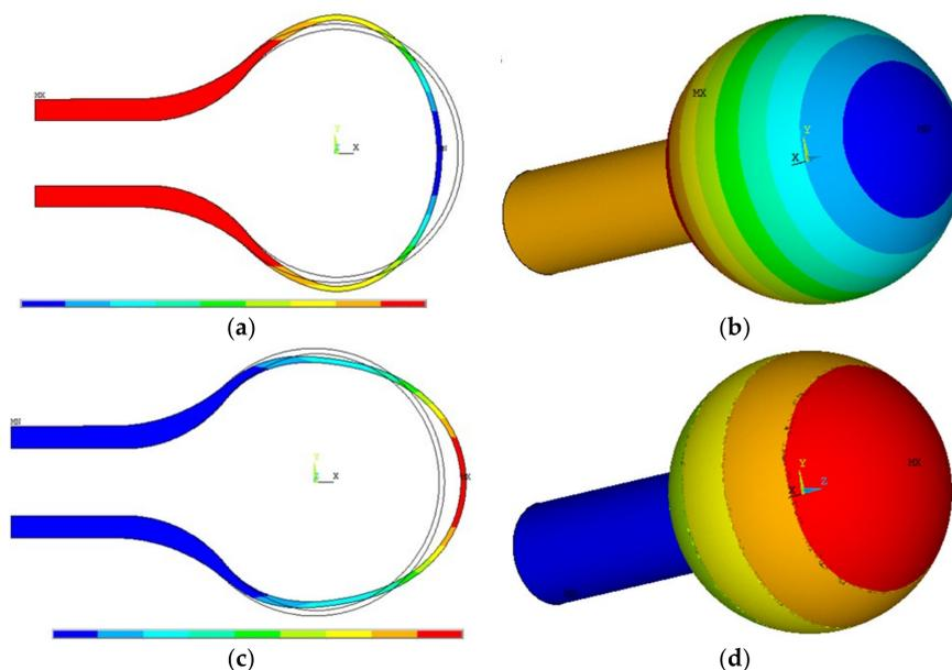
**Figure 11.** Deformation characteristic of the single-ended microbubble under the filling pressure of 4 and 1400 kPa. (a) Inner pressure: 4 kPa, 2D view; (b) inner pressure: 4 kPa, 3D view; (c) inner pressure: 1400 kPa, 2D view; (d) inner pressure: 1400 kPa, 3D view.
