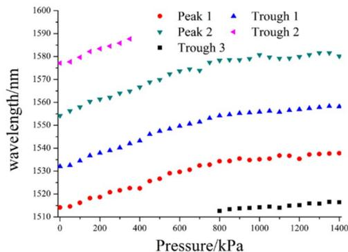
**Figure 7.** Relationship peak wavelength shift and filling pressure.
