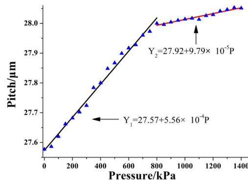
Figure 8. The relationship of pitch distance  $d$  and the filling pressure.
