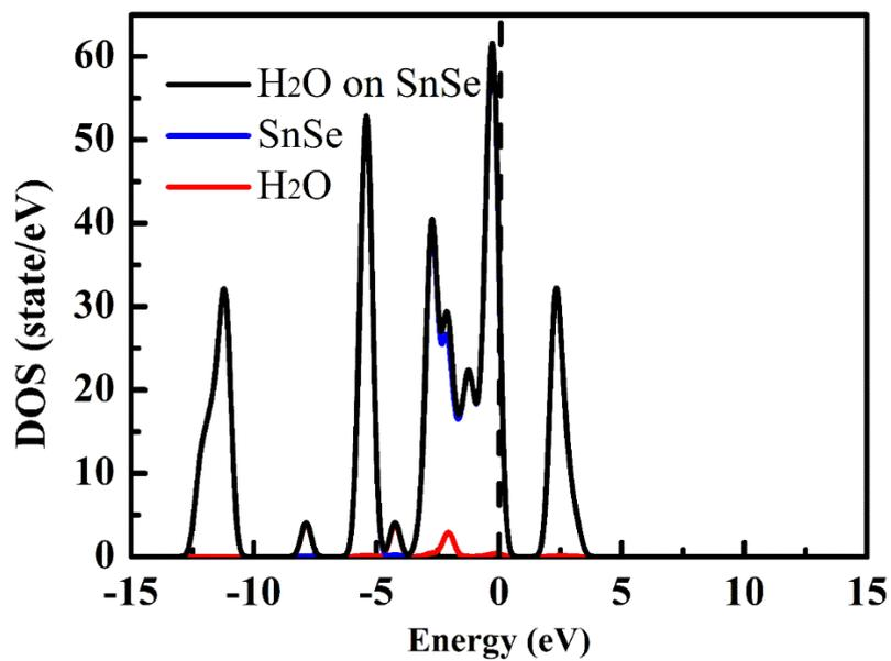
**Figure S4.** Total DOSs of the H<sub>2</sub>O on SnSe (black curve), the projected DOS of SnSe (red curve), and the adsorbate molecules (blue curve) for H<sub>2</sub>O on SnSe monolayer. The  $E_f$  is set to zero, as illustrated by black dotted line.
