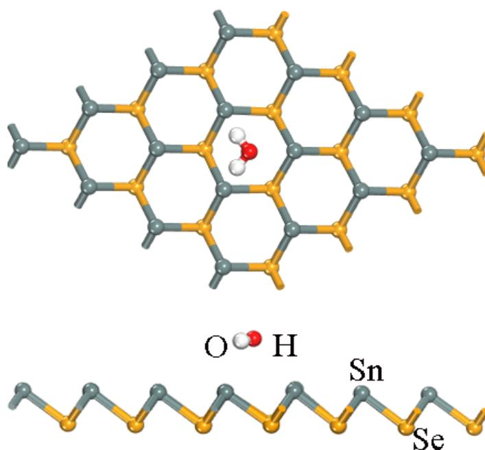
**Figure S2.** The most stable site of structural optimizations for H<sub>2</sub>O on  $\beta$ -SnSe layer is presented.
