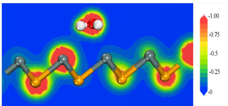
**Figure S5.** The slice of charge densities for the  $\beta$ -SnSe monolayer with the H<sub>2</sub>O molecule. The value of electron densities ranges between 0 and 1.00 e/Å<sup>3</sup>.
