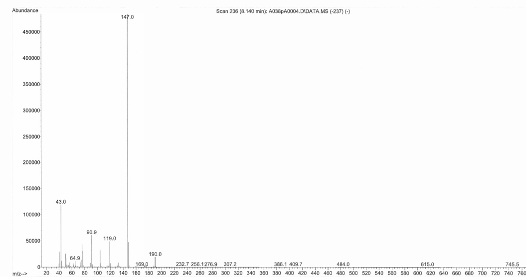
Figure S2. GC/MS chromatogram obtained for photocatalytic degradation of IBP (50 mg/L) under UVA irradiation, the identified degradation intermediates are shown in Table 2. (a) GC/MS chromatogram, (b) 4-Isobutylbenzaldehyde, (c) 4-Isopropylbenzaldehyde, (d) 4-Ethylacetophenone, (e) 4-Isobutylacetophenone, (f) 4-(1-carboxyethyl)benzoic acid.
